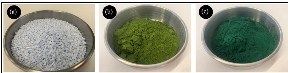
**Figure 2.** Materials used for filament production: (a) PETG granules produced by cutting and shredding Formfutura HDglass filament, (b) *Chlorella vulgaris* spray dried powder obtained from Algenium GmbH, (c) *Spirulina platensis* spray dried powder from Algenium GmbH
