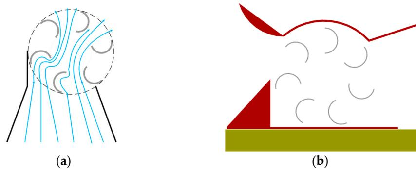
**Figure 13.** (a) 6-blade CFWT with converging nozzle and (b) the CFWT with diffuser-shaped shroud.
