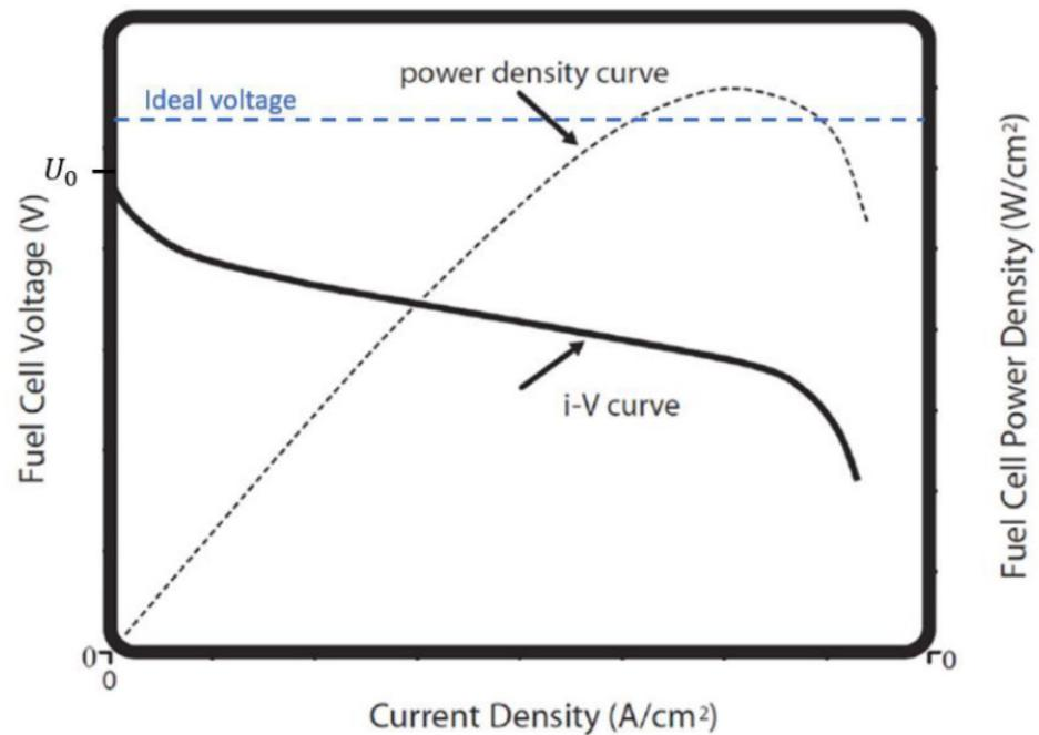
Figure 2. Current-voltage and power-density curve of a fuel cell.
