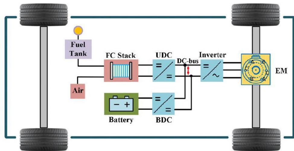
Figure 7. Powertrain of an FCHEV with parallel configuration.
