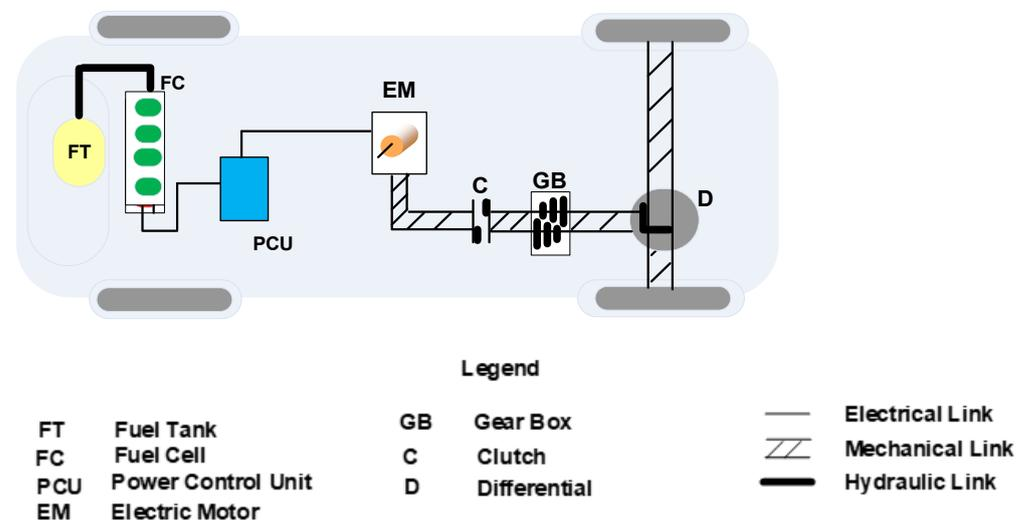
**Figure 5.** Fuel cell electric vehicle and its components.
