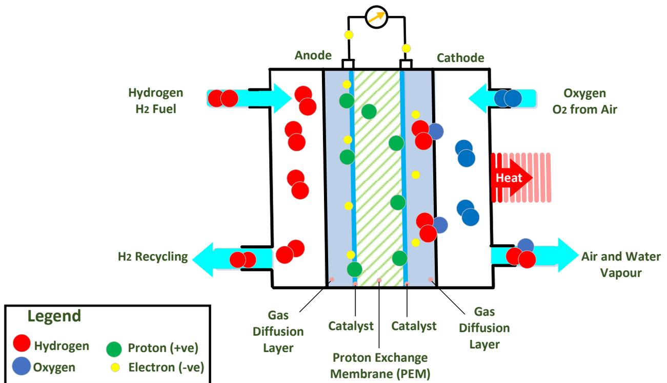
**Figure 1.** The basic concept of hydrogen fuel cell.
