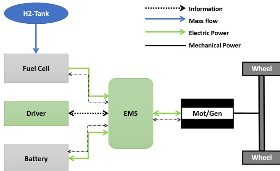
Figure 8. Simplified powertrain structure of an FCHEV in a parallel hybrid configuration.
