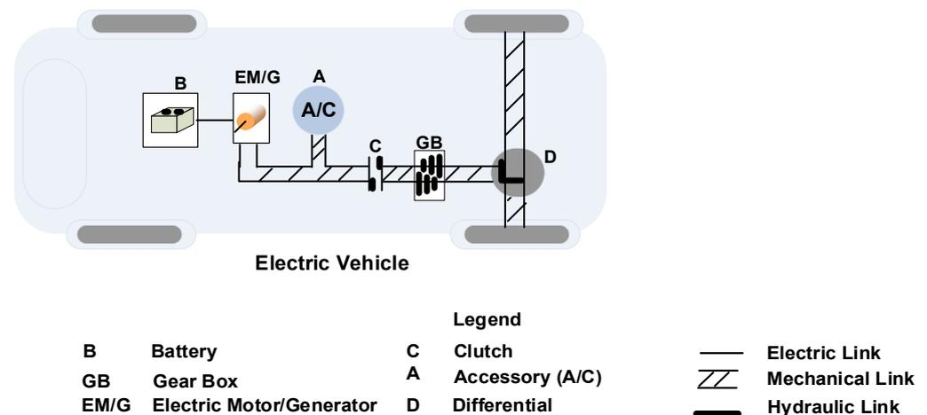
**Figure 4.** Electric vehicle and its components.
