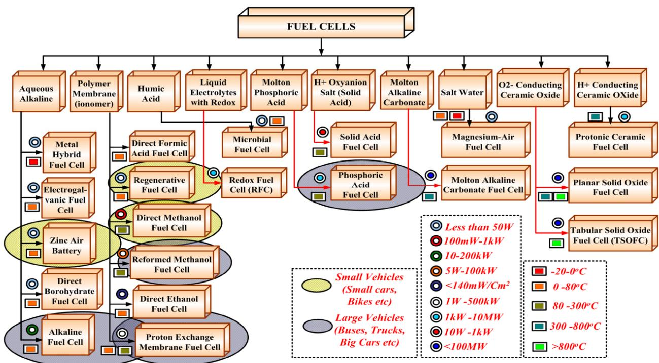
Figure 3. Classification of Fuel Cell (based on the type of electrolyte, power, and working temperature) [28].
