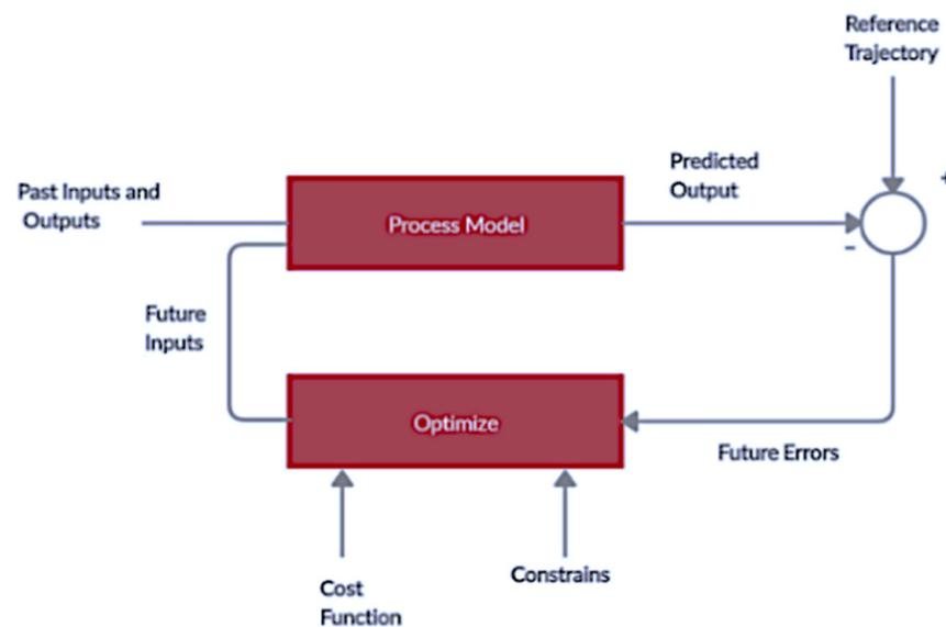
Figure 11. Block diagram of MPC-based EMS.
