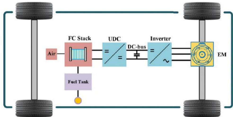
**Figure 6.** Powertrain configuration of a FCEV.
