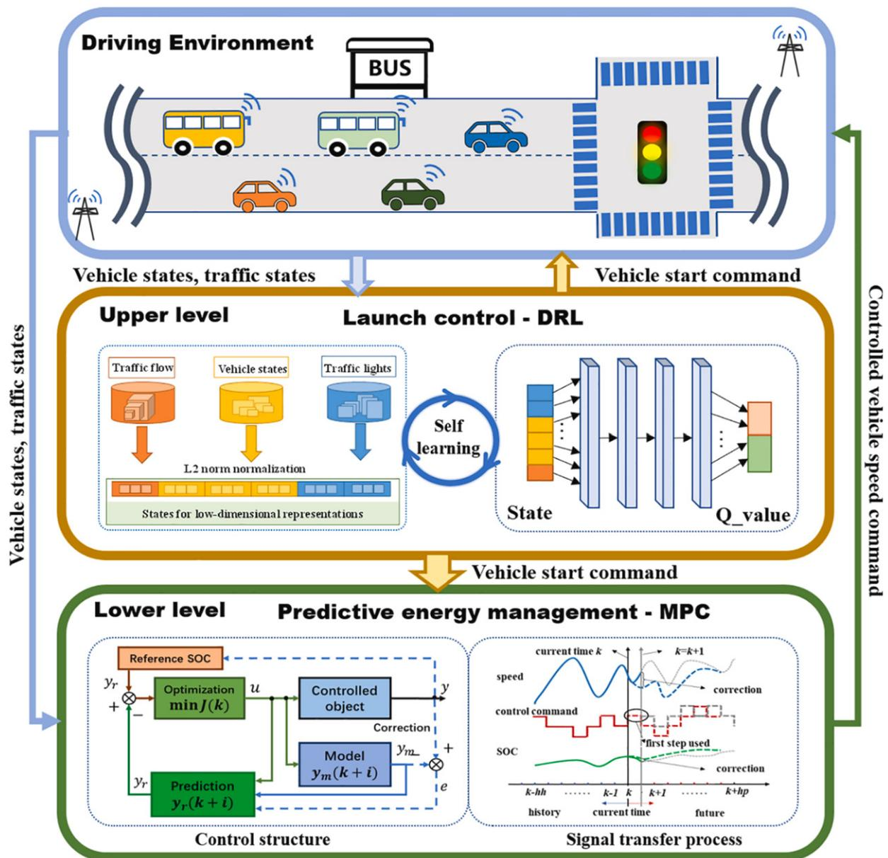
**Figure 12.** Novel dual-layer Energy management system that utilizes both internal system parameters as well as traffic information to optimize the vehicle operation strategy proposed by Yan et al. [162].
