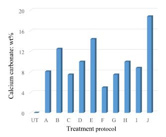
**Figure 9.** Relative performance of EICP treatment protocols in terms of calcite precipitation. Refer to Table 1 for summaries of the treatment protocols.
