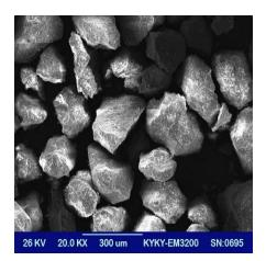
Figure 1. Scanning electron microscope (SEM) image of untreated (UT) test sand.
