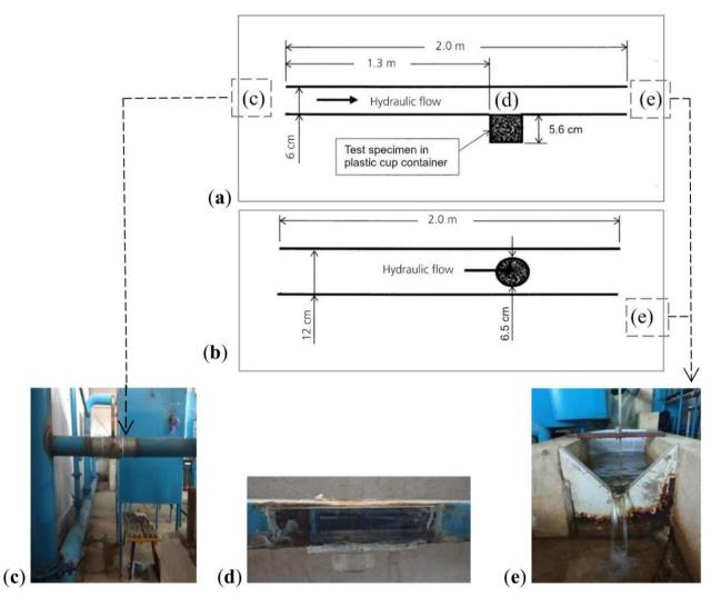
velocity values, measuring the times required to erode and remove the protruding 1-mm tall sand layer when subjected to three different tangential shear stress.
