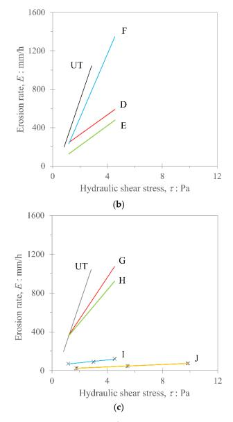
**Figure 10.** Erosion charts for various EICP treatments: (a) protocols A–C; (b) protocols D–F; (c) protocols G–J (refer to Table 1 for descriptions of the different protocols). Note: UT, untreated sand.
