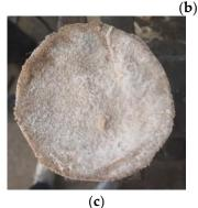
**Figure 5.** (a) Specimen container fitted with side drainage port and plastic-film extension collar fitted around top rim. (b,c) side and top views of white calcite deposits visible on surface of 14-day cured EICP-treated sand specimen.
