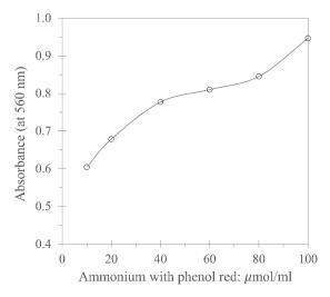
**Figure 3.** Calibration plot for change in absorbance at a wavelength of 560 nm measured by spectrophotometer.
