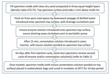
Figure 2. Flow chart of specimen making process.
