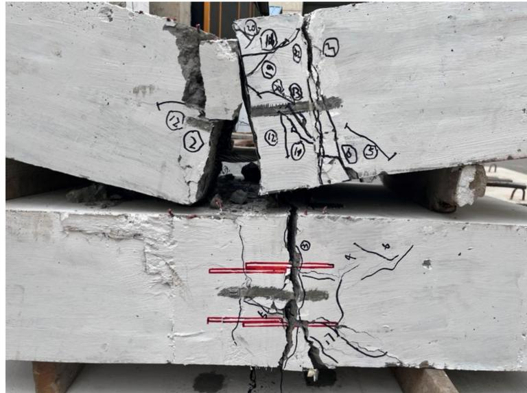
**Figure 9.** The seismic RC beams in the earthquake simulation laboratory.
