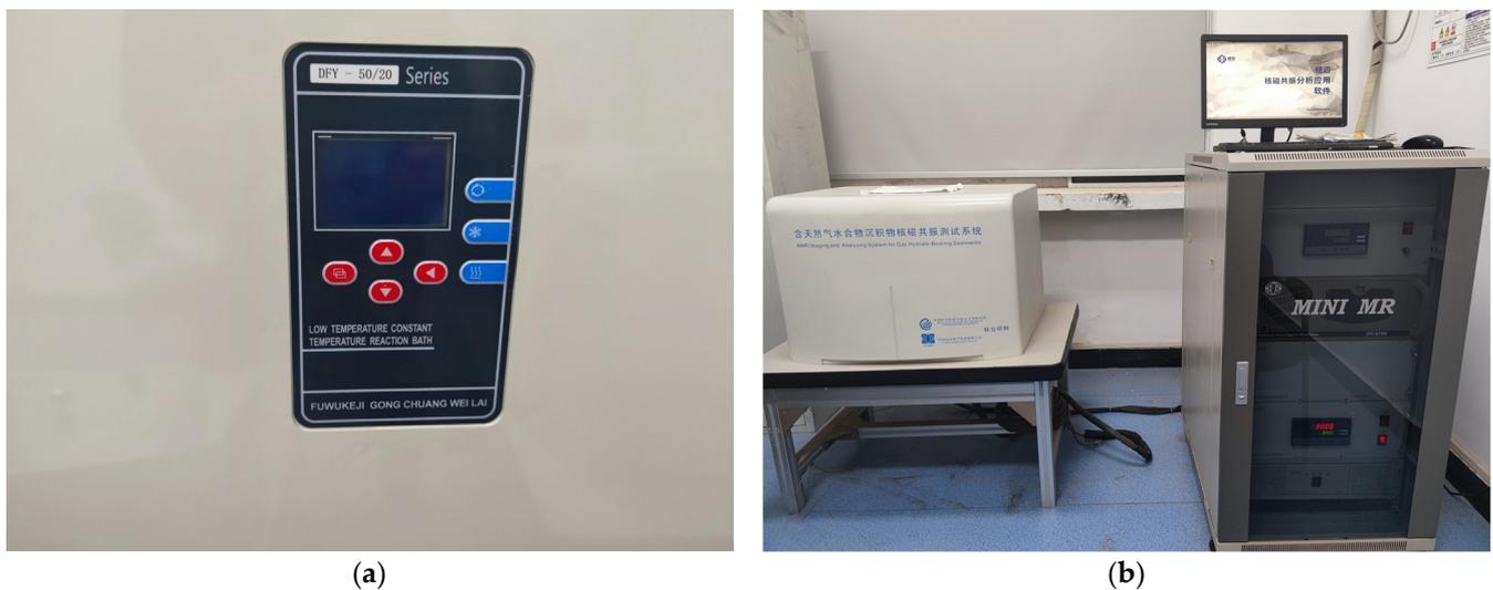
**Figure 2.** Experiment instruments. (a) Cold bath device; (b) Nuclear magnetic resonance instrument.
