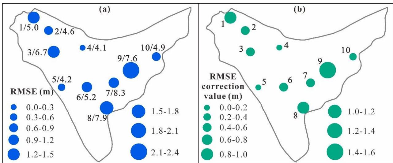
**Figure 7.** Spatial distribution of *RMSE*s and *RMSE* correction values for 10 wells during the prediction period. Note: (a) *RMSE* of the GWLs predicted by the MODFLOW model; (b) *RMSE* correction value; *RMSE* correction value = *RMSE* of MODFLOW model – *RMSE* of LSTM2 model. Numbers 1 to 10 correspond to wells numbered 1 to 10, respectively; “1/5.0” represents the well numbered 1 and the overall range of GWL variation for this well from January 2015 to May 2019.
