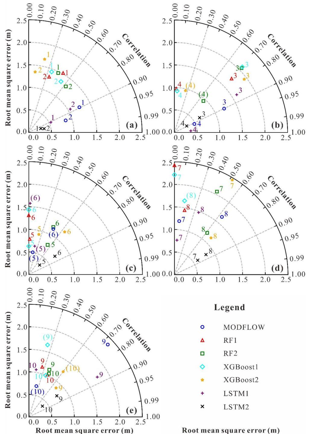
**Figure 4.** Taylor diagram of PR and RMSE for 10 wells at prediction periods based on different models. Note: (a) describes wells numbered 1 and 2; (b) describes wells numbered 3 and 4; (c) describes wells numbered 5 and 6; (d) describes wells numbered 7 and 8; and (e) describes wells numbered 9 and 10. The well numbers in parentheses indicate negative PR values, with the absolute value used instead.
