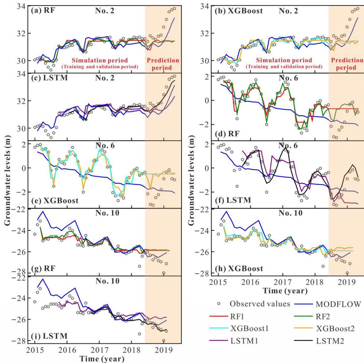
**Figure 5.** Comparison of simulated dynamic GWL curves for 3 wells based on different models. Note: Simulation period includes training period and validation period; No. 2, No. 6, and No. 10 represent wells numbered 2, 6, and 10, respectively; (a,d,g) represent the dynamic GWL curves plotted by the RF1 and RF2 models; (b,e,h) represent the dynamic GWL curves plotted by the XGBoost1 and XGBoost2 models; and (c,f,i) represent the dynamic GWL curves plotted by the LSTM1 and LSTM2 models.
