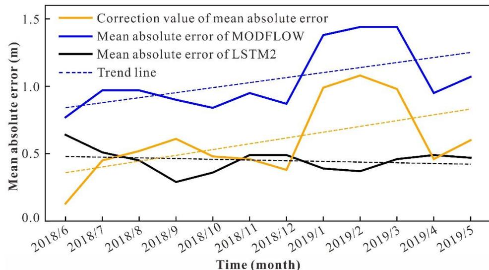
**Figure 6.** Variation curves of correction value of mean absolute error over time for LSTM2 model during the prediction period. Note: Correction value of mean absolute error = mean absolute error of MODFLOW model – mean absolute error of LSTM2 model.
