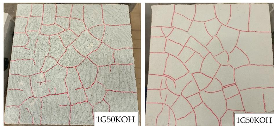
Figure 13. Observed restrained shrinkage of the KOH at 21 days.
