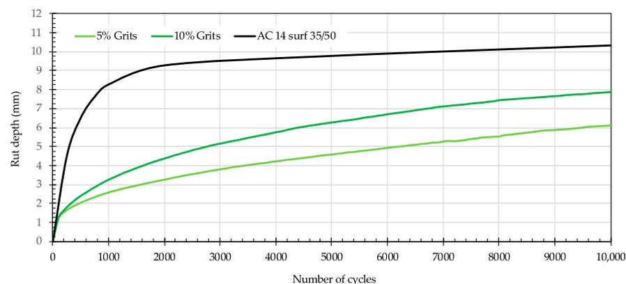
**Figure 11.** Variation of rut depth in wheel-tracking test results.
