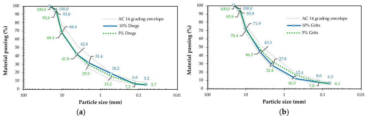
Figure 4. Gradation of the aggregate’s blend: (a) with dregs; (b) with grits.
