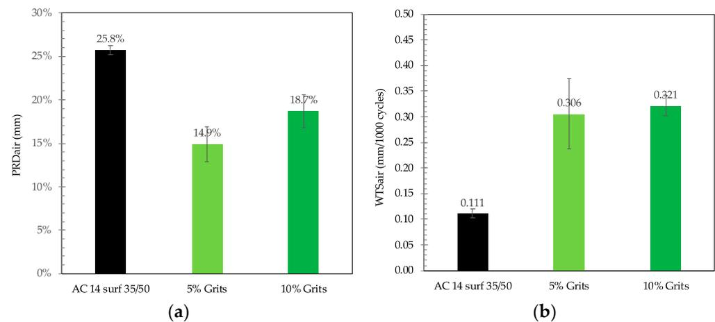
**Figure 12.** Results derived from wheel-tracking curves: (a) PRD<sub>air</sub>; (b) WTS<sub>air</sub>.
