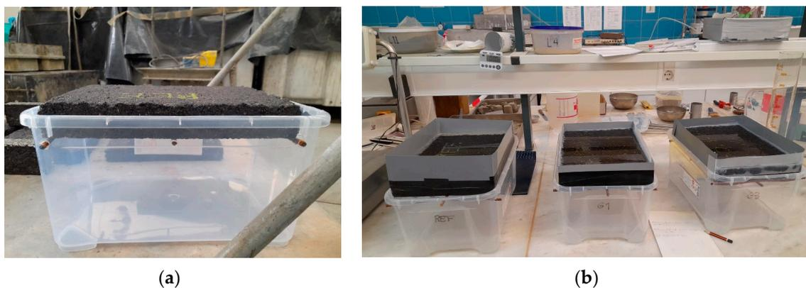
**Figure 7.** Water load test: (a) detail of the supporting box and its slab; (b) testing procedure.
