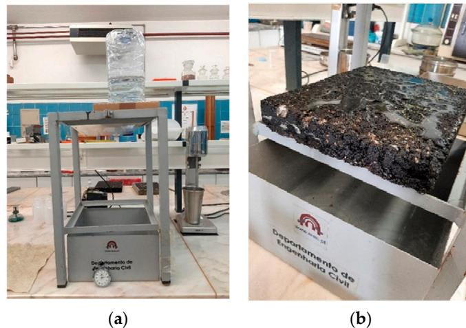
Figure 8. Surface runoff tests: (a) water raining system; (b) surface runoff detail.
