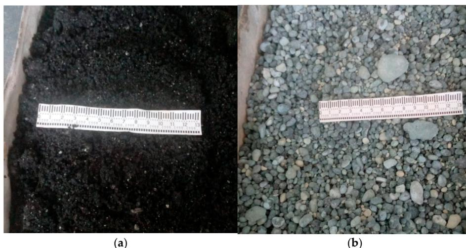
**Figure 1.** Samples of dregs (a) and grits (b).
