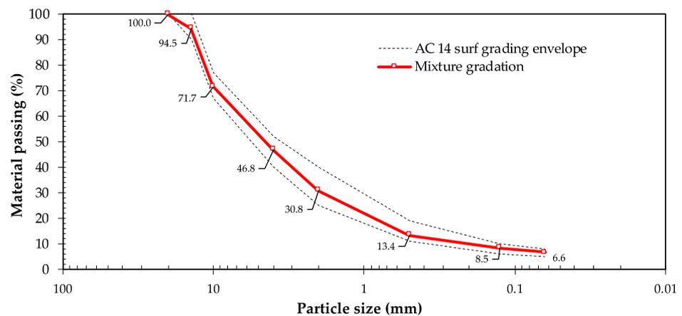
Figure 3. Gradation of the aggregate’s blend and grading envelope requirements.
