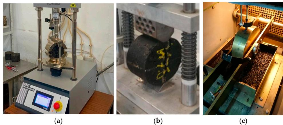
**Figure 6.** Laboratory tests to evaluate mechanical properties: (a) Marshall test; (b) indirect tensile strength; (c) wheel-tracking test.
