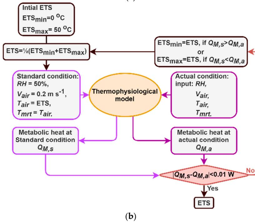
**Figure 2.** (a) Dynamic simulation processes of the 2-node model; (b) schematics of algorithm to obtain the ETS using the 2-node model.
