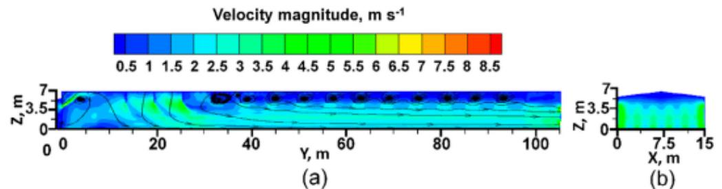
**Figure 3.** Airflow streamlines and air speed distribution for the (a) longitudinal section and (b) cross-section in the hen house with ceiling deflectors.
