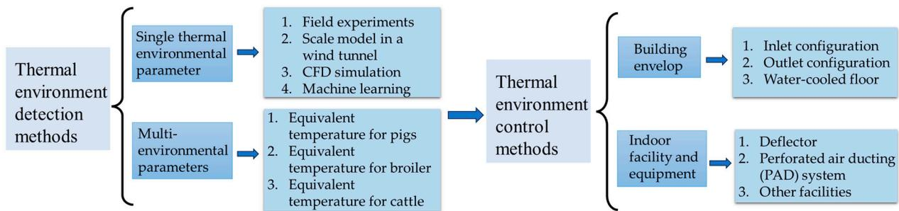
**Figure 1.** Flowchart of relationship between the detection and control methods.
