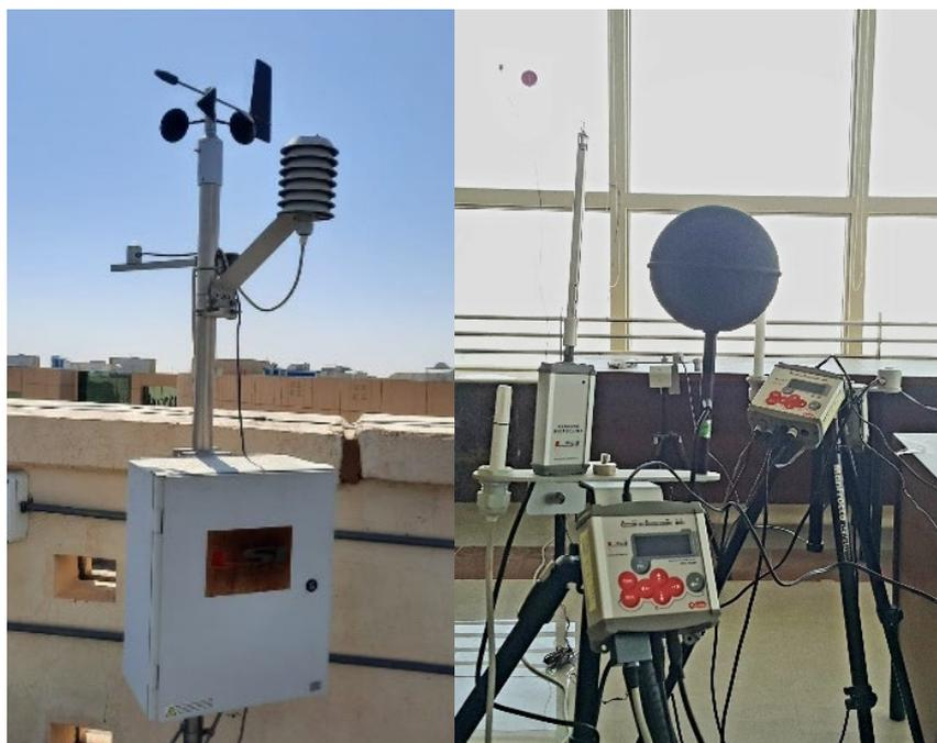
**Figure 6.** Data loggers for indoor and outdoor environments (LSI-R-Log and LSI-E-Log Weather Station).
