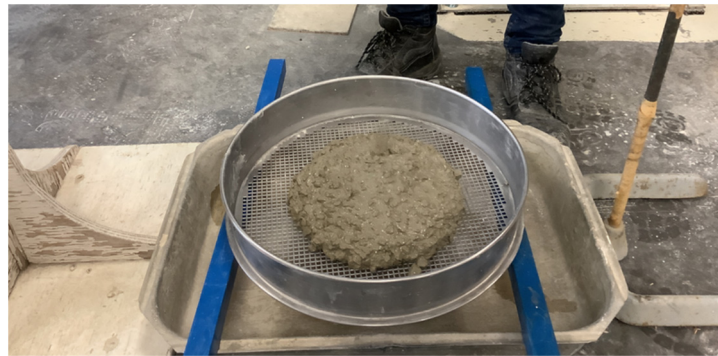
Figure 3. SCC under sieve analysis test.
