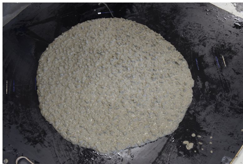
Figure 4. SCC under slump-flow test.
