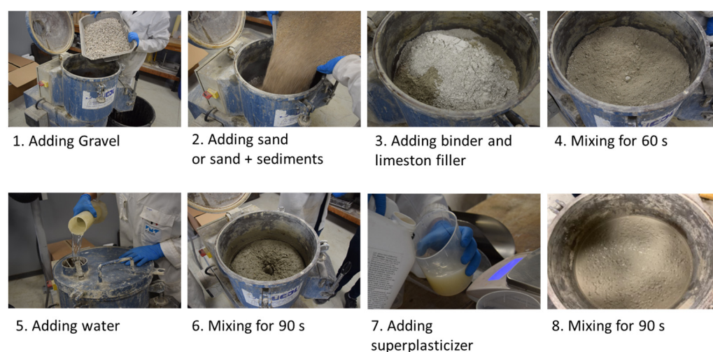
Figure 2. Self-compacting concrete preparation process.
