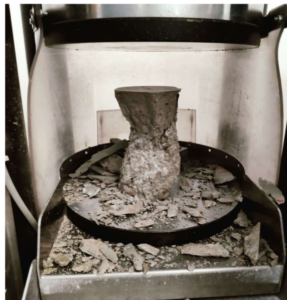
Figure 5. SCC at 28 days under Compressive strength test.
