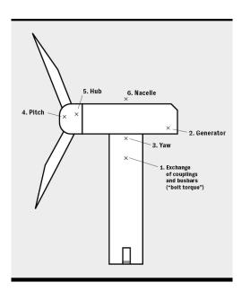
**Figure 2.** Representation of a wind turbine with all the "critical points" collectively identified by the O&M technicians.
