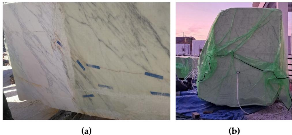
**Figure 4.** Resining marble blocks inside the CMB; (a) resining a block directly in the quarry by external consolidation and “stitching” the fractures; (b) resining a block in working plants by the vacuum method (resin is also injected inside the block), applied before cutting into slabs, to obtain as many slabs as possible at the final stage.
