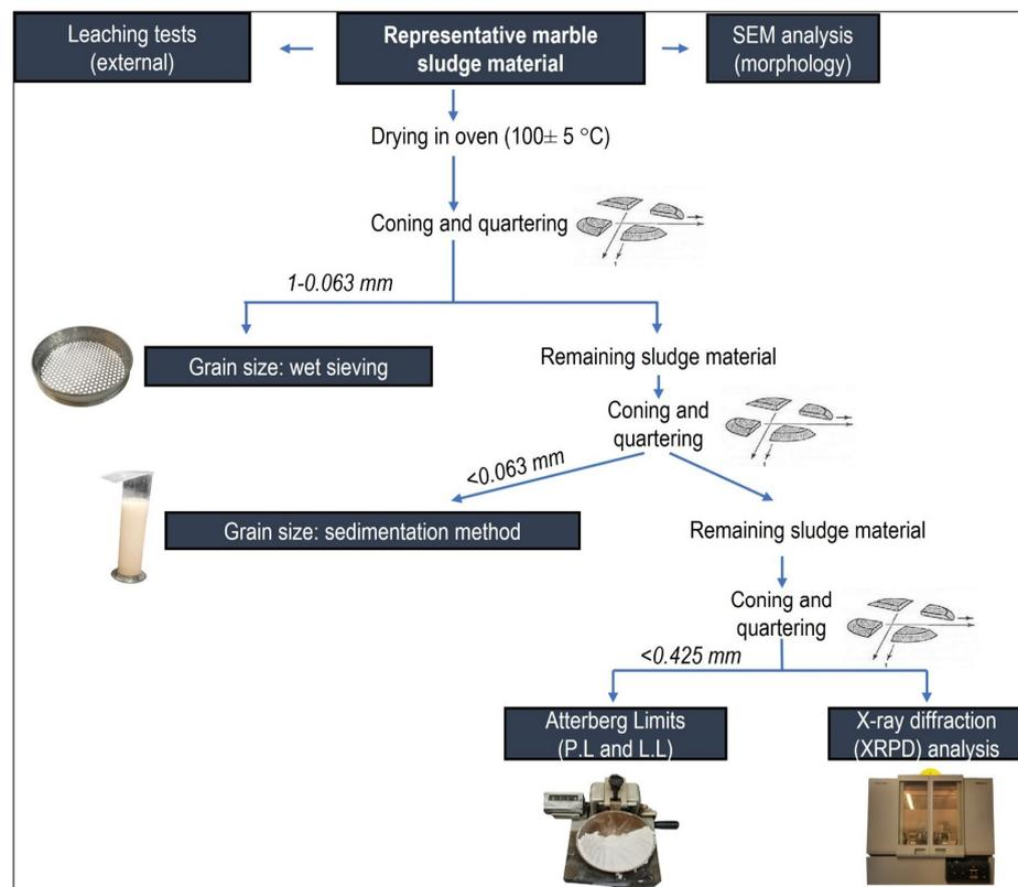
**Figure 10.** Analytical procedures on Carrara marble sludge samples.
