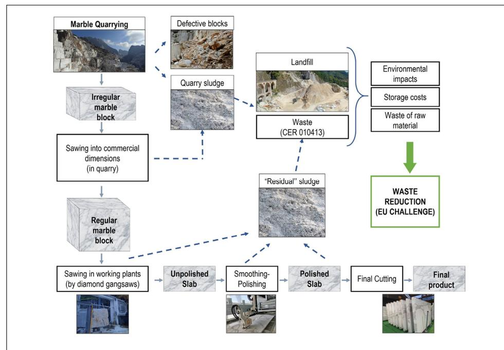
**Figure 7.** Schematic overview of marble quarrying and processing activities (continuous blue lines) with a focus on sludge (quarry sludge and residual sludge) generation (dotted blue lines) and management issues (green arrow).
