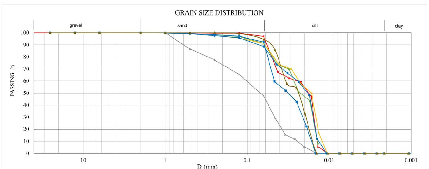
**Figure 11.** Grain size characteristics of Carrara marble sludge samples (grey line: marble sludge from chainsaw cutting—in quarry; sludge from diamond wire cutting—in quarry; blue lines: sludge from processing and marble squaring—in quarry; green line: sludge from processing and marble squaring—in working plant; red line; brown and yellow lines: filter pressed/dewatered sludge—in working plant and processing facilities).
