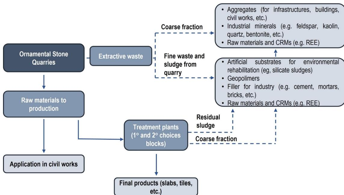
**Figure 1.** Simplified flow diagram about potential recovery of EW from dimension stones (modified from [26]).
