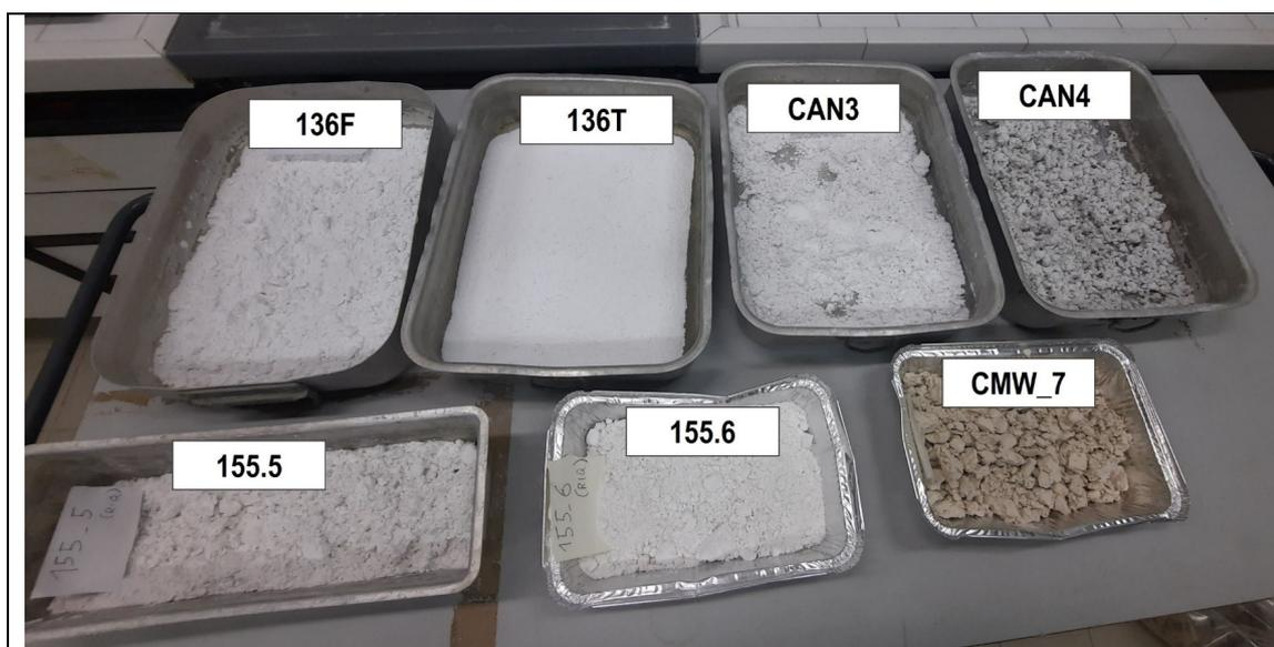
**Figure 9.** Representative samples of Carrara marble sludge in the laboratory.
