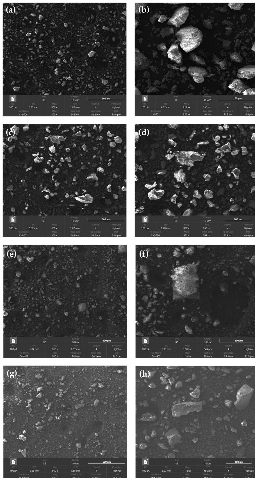
**Figure 13.** SEM images of calcium carbonate grains in the Carrara marble sludge: (a,b) marble quarry sludge from diamond wire machine cutting; (c,d) marble quarry sludge from chainsaw machine cutting; (e–h) sludge from treatment operations (filter-pressed sludge in working plant and recycling facilities).
