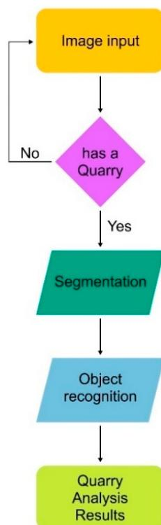
**Figure 1.** Workflow of the process developed for the aggregates quarry detection.
