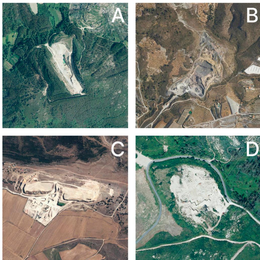
**Figure 2.** Examples of different types of active aggregates quarries. (A) Quarry located within a forest in the north of Spain, with a restored zone on the left side of the quarry. (B) Quarry in a dryland area in the south of Spain. (C) Quarry near a hill, in the central part of Spain. (D) Quarry for ornamental rocks (aggregates are in this case a by-product).
