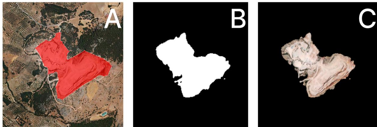
**Figure 3.** Process of segmentation of an aggregate quarry. (A) Satellite image where a quarry has been digitized. (B) Mask calculated with the machine learning model. (C) The aggregates quarry resulting from clipping the satellite imagery with the mask proposed by the model.
