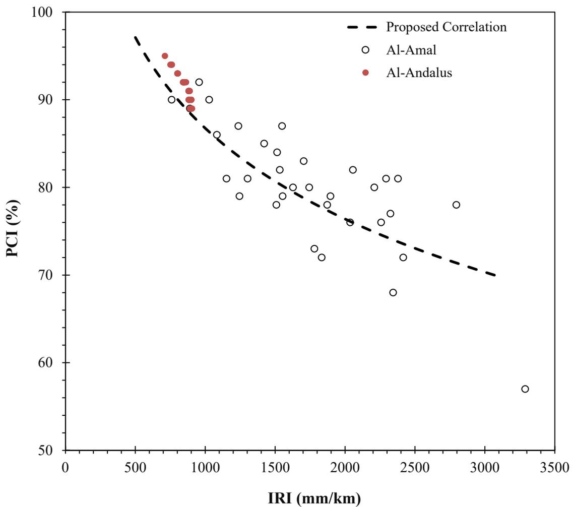
Figure 10. PCI and IRI validation values for Al-Amal and Al-Andalus roads versus the proposed correlation.
