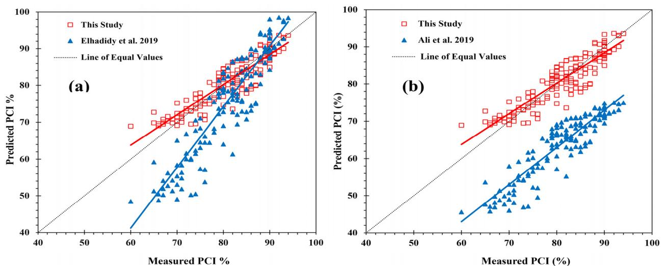
**Figure 11.** Comparison with reported prediction models performed by (a) Elhadidy, El-Badawy, and Elbeltagi [4] and (b) Ali, Hossain, Hussein, Swarna, Dhasmana, and Hossain [2].
