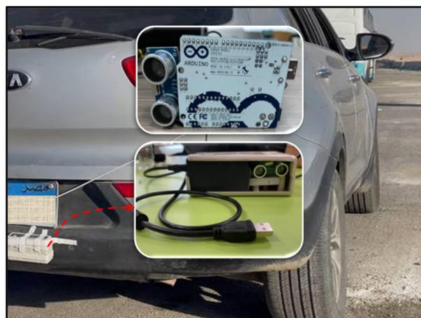
**Figure 5.** Mobile ultrasonic distance sensor mounted to a vehicle to estimate IRI values (Arduino board connected to the sensor and housed for mobile data collection).
