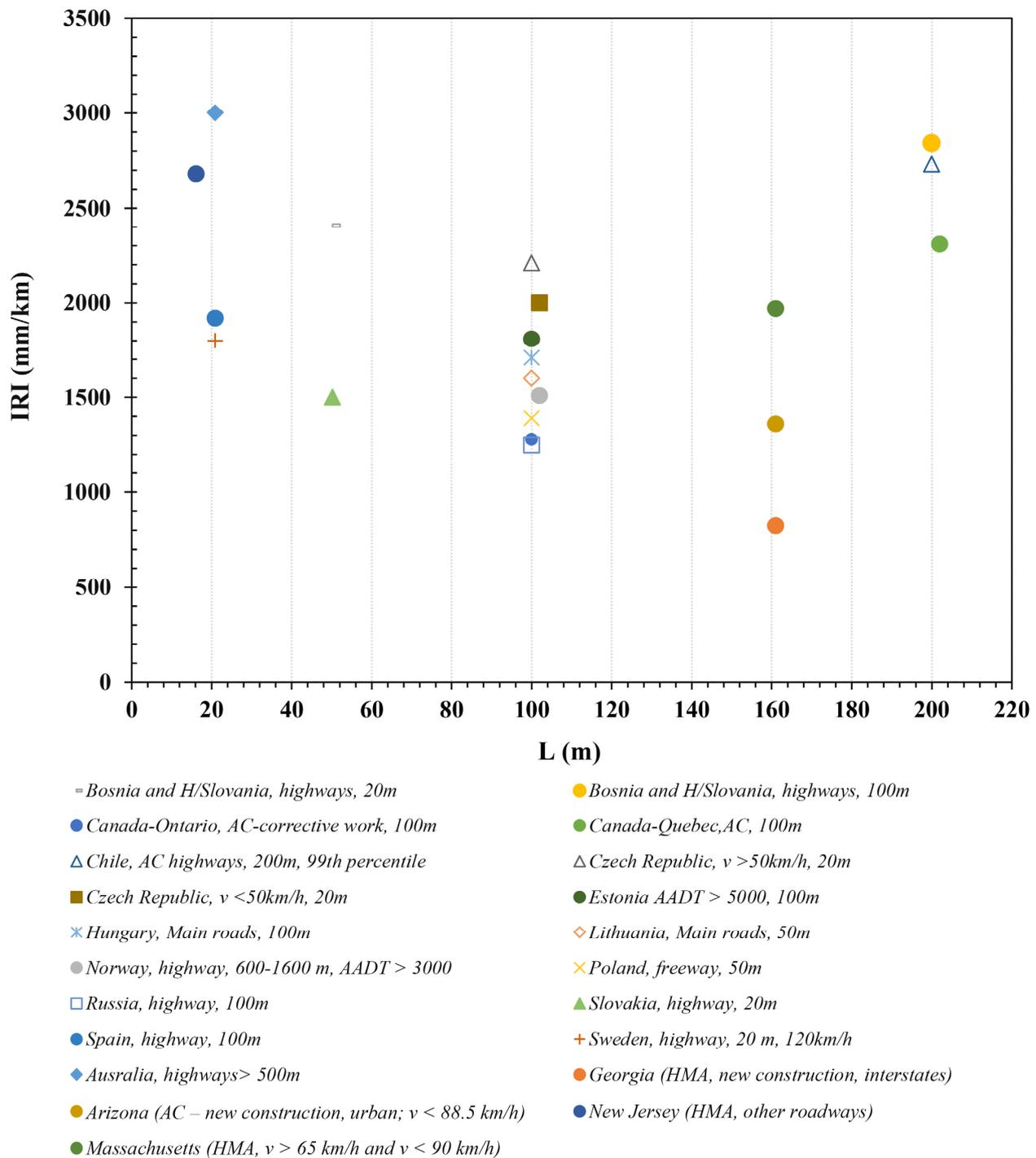
**Figure 1.** IRI limit values for new or reconstructed roads as a function of segment length (L). (after [25]).
