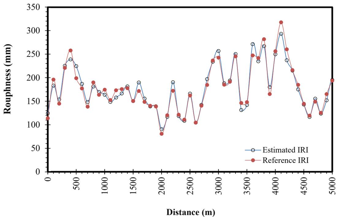
**Figure 6.** Road surface deformation (average irregularities in wheel paths shown in absolute value) for a 5 km stretch of Ashabab Road for both estimated and reference IRI values.
