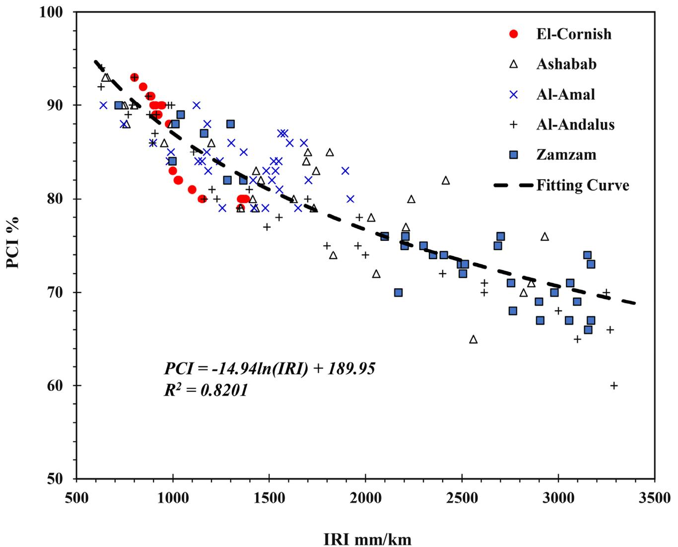
**Figure 8.** Proposed correlation for the collected IRI and PCI values.
