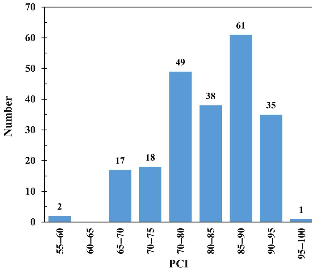
**Figure 7.** Distribution of the calculated PCI values (221 data points) for the roads of the study area.
