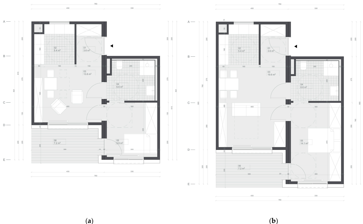
Figure 3. Dwelling unit plans created and evaluated by authors: (a) dwelling unit for one, unit area 39.2 m 2 and a balcony of 7 m 2 ; (b) dwelling unit for two, unit area 49.3 m 2 and a balcony of 7 m 2 .
