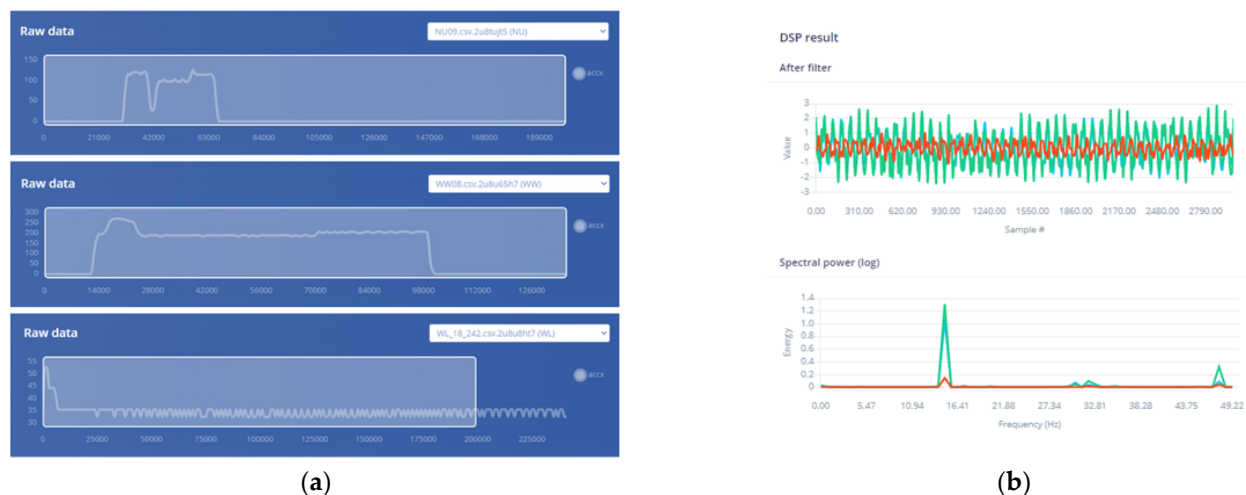
Figure 6. (a) Water flow sample data used for training the smart faucet system model; (b) Accelerometric sample data used for training the water-pump malfunction-detection system model.
