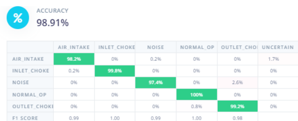
Figure 7. (a) Estimated performance of the machine-learning model for the smart faucet system; (b) Equivalent results for the water-pump malfunction-detection model.
