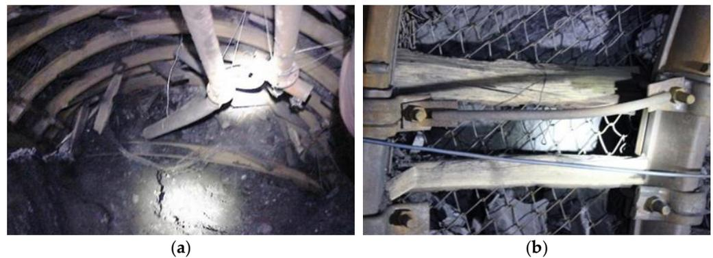
**Figure 14.** Destruction of U shape support. (a) Anchor rod failure situation, (b) anchor network damage situation.
