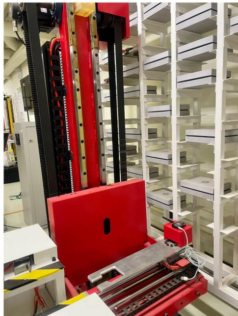
**Figure 4.** Image of stacker robot.
