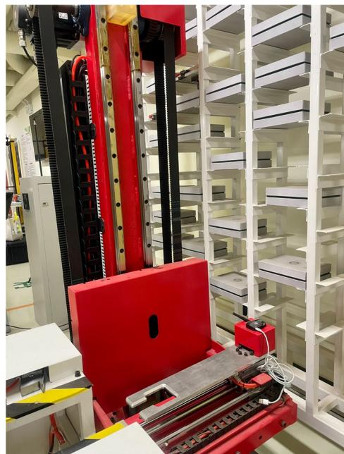
**Figure 4.** Image of stacker robot.
