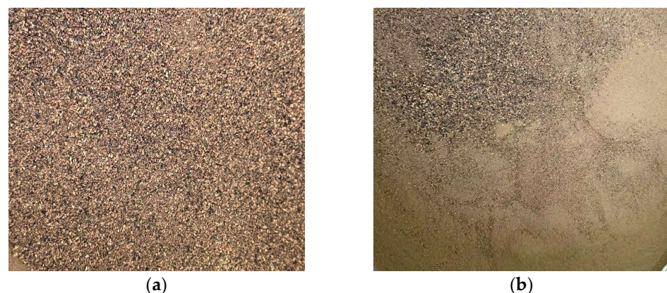
Figure 7. The SGS images of the 0–0.6 mm and 0.6–1.18 mm particle size ranges: (a) 0.6–1.18 mm, (b) 0–0.6 mm.
