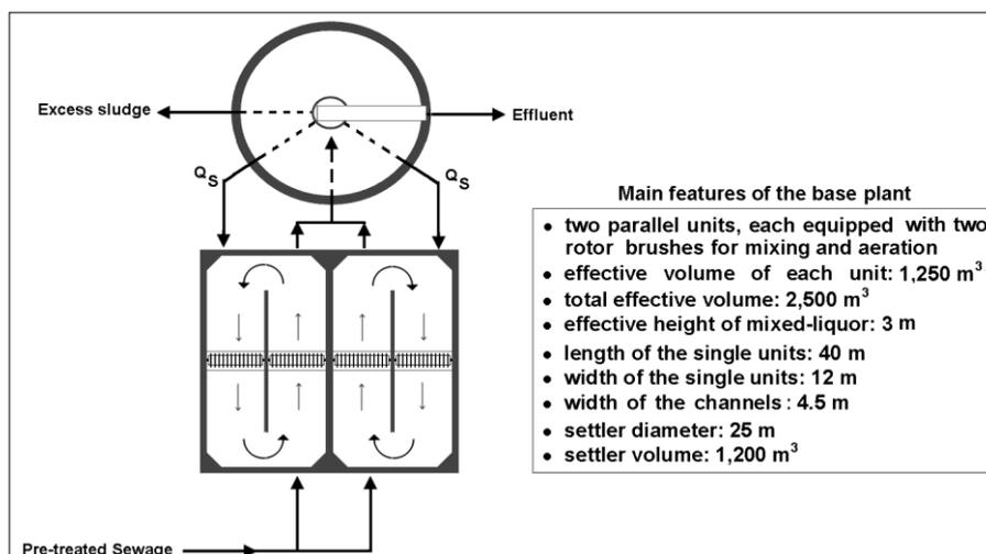
This base plant was modified in order to obtain the two alternative processes shown in Figure 2:
