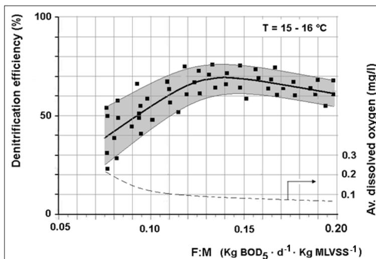
**Figure 6.** Efficiency of denitrification in the simultaneous process (Scheme B).
