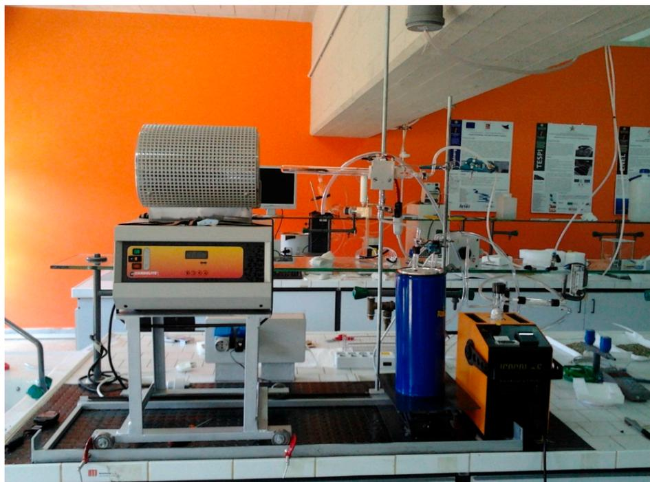
The system consists of a quartz cylindrical reactor 340 mm long and 20 mm internal diameter closed at one end and provided with a 29/32 mm open end. The reactor body is provided with an 8 mm diameter side-connection to sweep the pyrolysis products away.
