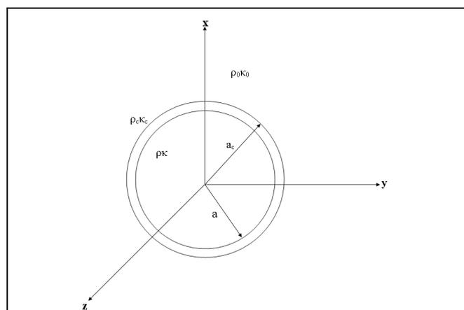
Pressure and radial velocity continuity at the interfaces have to be applied, giving rise to a  $4 \times 4$  linear system to be solved as a function of the scattering coefficients, which, in turn, depend on the cover elastic properties,  $\rho_c$  and  $\kappa_c$ .
