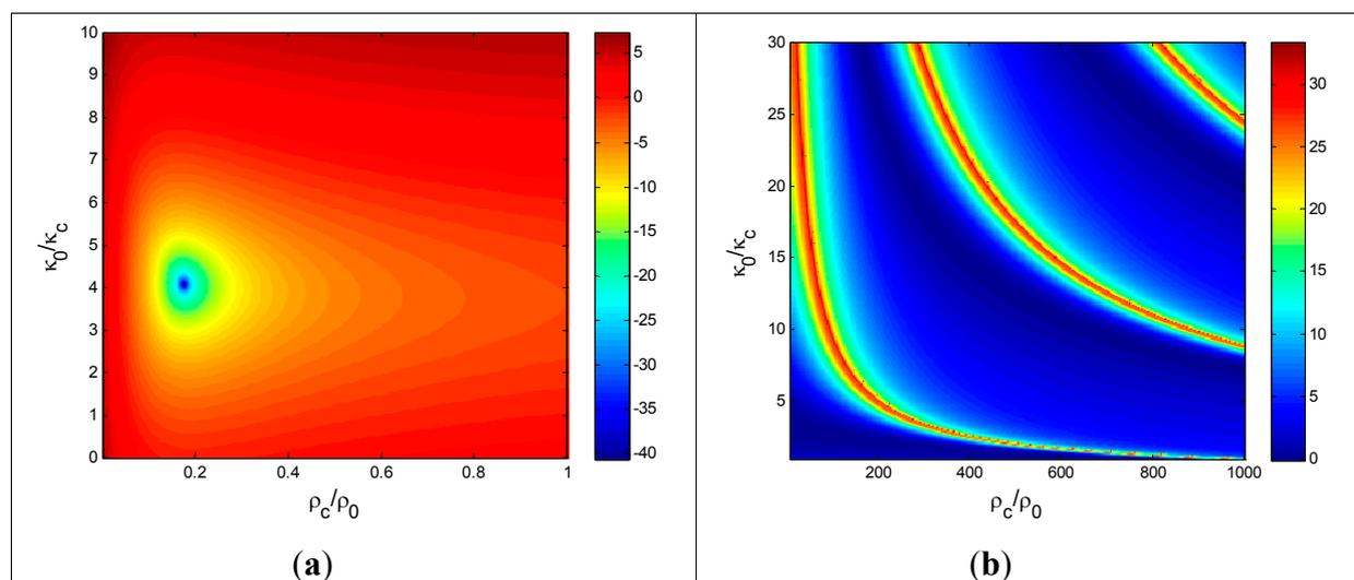
We therefore focus on the plasmonic scattering region and analyze the sensitivity of the SCS to parameter variations for different coating thicknesses ( $a_c = 1.1a$  and  $1.5a$ ) and sphere dimensions ( $k_0 a = 0.1, 0.5$  and  $1.0$ ). All of these cases satisfy the condition of object smaller than the wavelength of the impinging wave.
