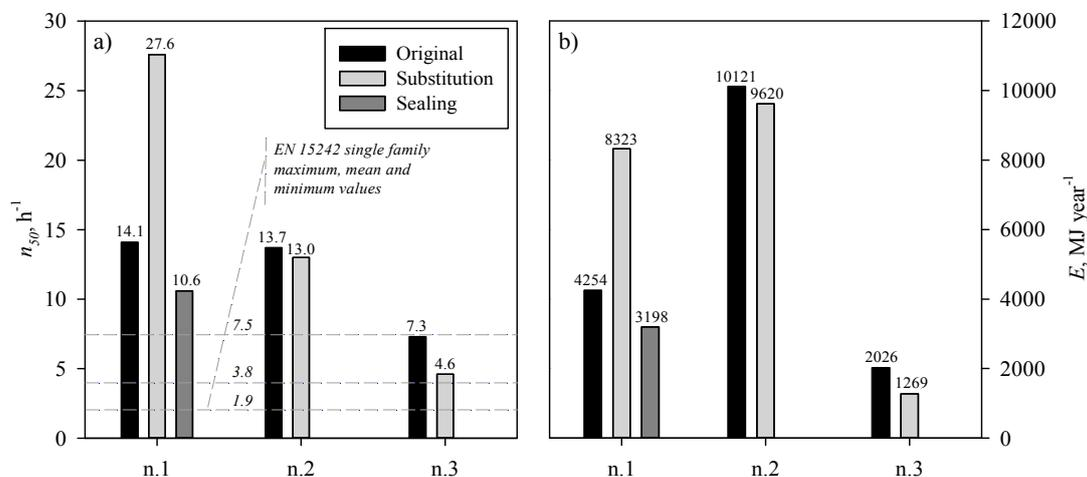
**Figure 1.** Comparison between: (a) experimental  $n_{50}$  and corresponding values of EN 15242 Standard; (b) actual energy demand for the three buildings.
