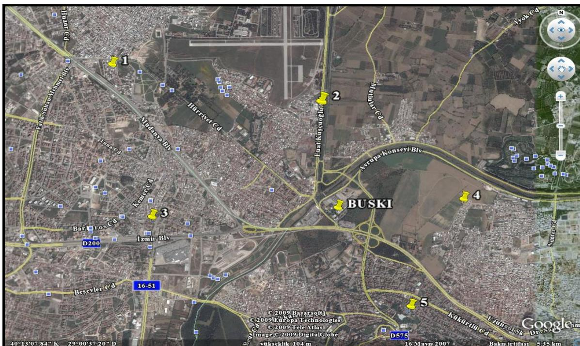
The static GPS observations were first carried out in the network with five sessions each comprising 30 minutes of observations made with three Zeiss GePos Experience™ GPS receivers. The same points were then measured with RTK GPS approach, and the differences between these two approaches are tabulated on the basis of differences in each coordinate axes in Table 4.
