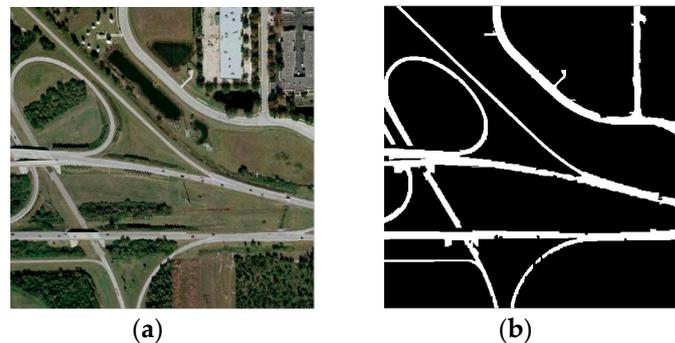
**Figure 2.** The extraction of initial road. (a) Original image; (b) Initial road after multiscale segmentation and feature extraction.
