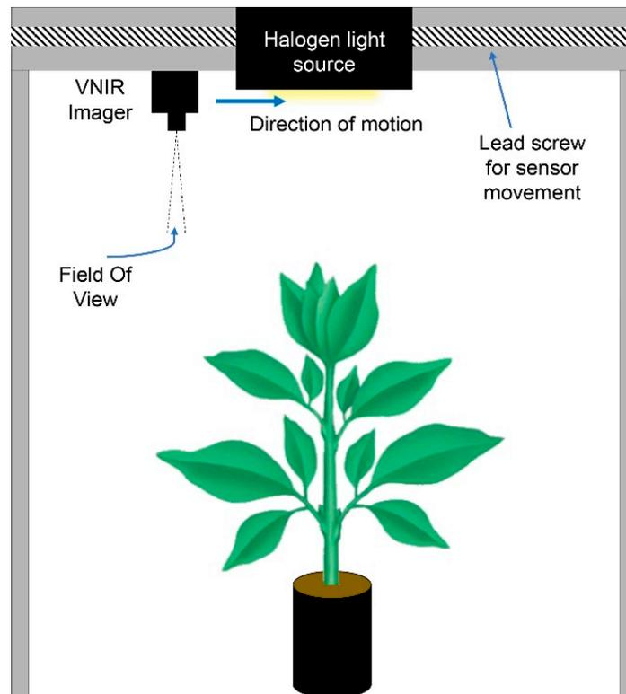
**Figure 1.** Schematic of the 3-m tall custom-built gantry system for sensor movement. The sensor is moved along a defined track by a lead screw. The halogen light source provides full spectrum artificial illumination for the object.
