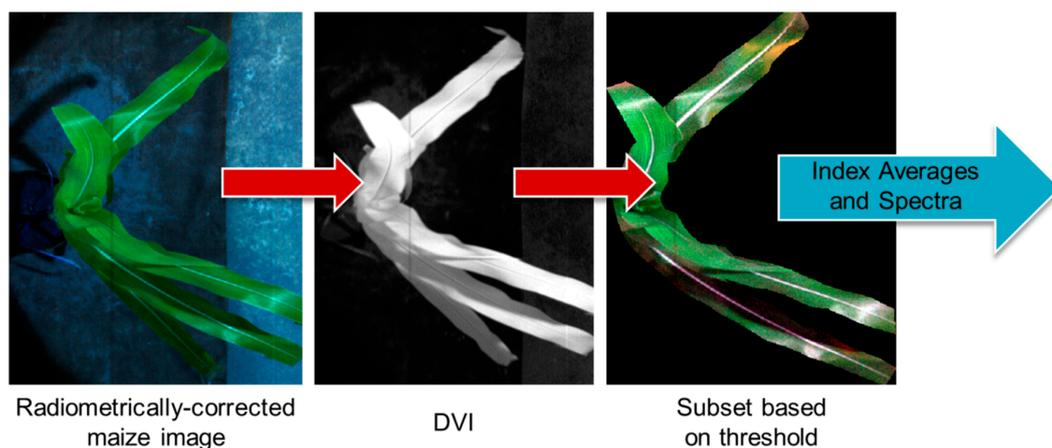
**Figure 2.** Image processing workflow. The Difference Vegetation Index was used to create a mask on radiometrically-corrected images with a threshold of values. Once masked, reflectance indices are only calculated and averaged on parts of images containing vegetation. Reflectance Index averages and reflectance spectra were then output for statistical analyses. Indices and spectra were averaged pixel-by-pixel for each image.
