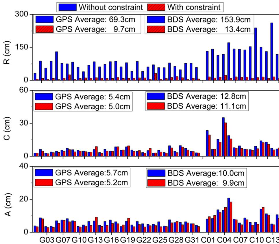
**Figure 4.** RMS of GPS and BDS orbit differences in the radial, cross-track and along-track directions of the clock-constrained and traditional RPPP POD solutions with respect to the dynamic POD solution.
