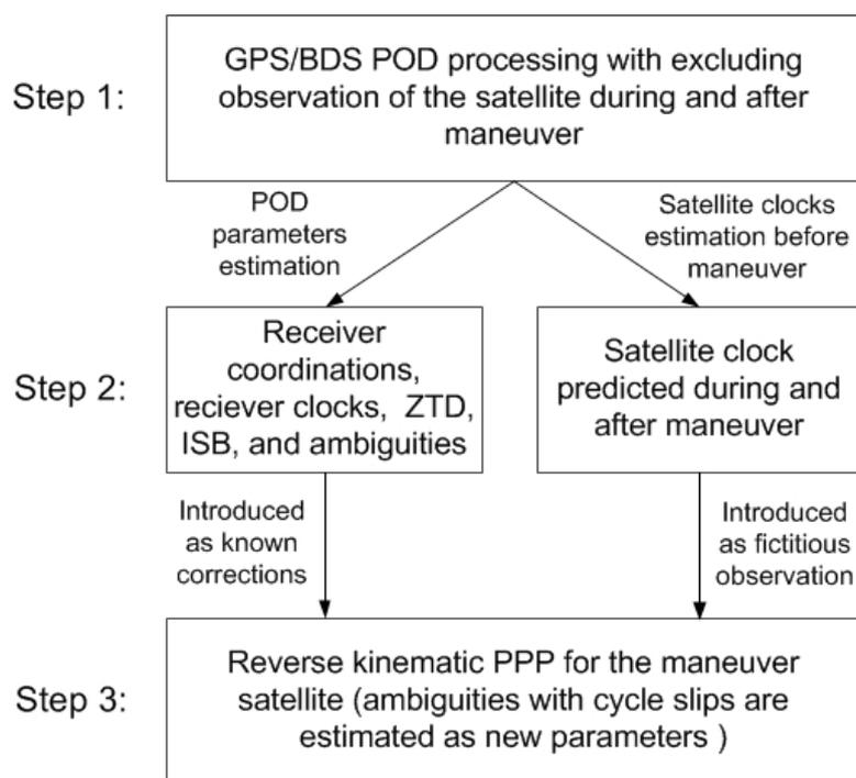
**Figure 2.** Processing scheme of the clock-constrained reverse precise point positioning (RPPP) precise orbit determination (POD) strategy for maneuvering satellites. GPS—global positioning system; BDS—Beidou navigation satellite system; ZTD—zenith tropospheric delays; ISB—inter-system bias.
