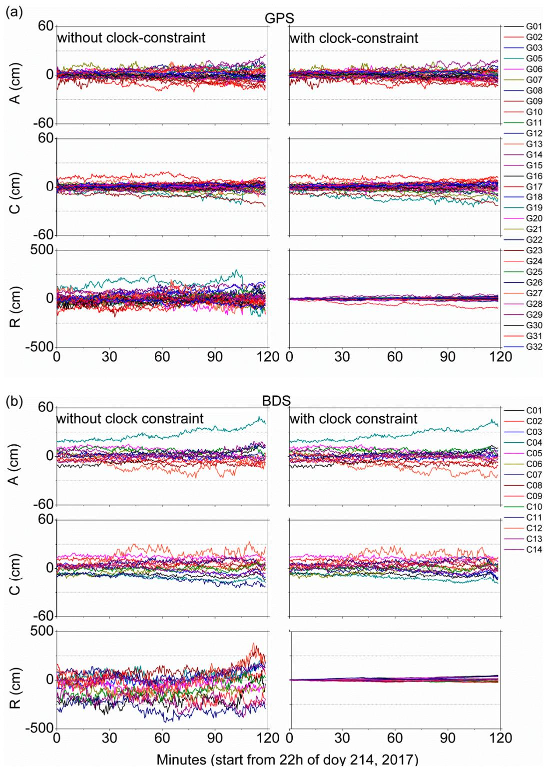
**Figure 5.** Orbit differences between the RPPP and dynamic POD solutions for GPS and BDS satellites ((a): Orbit differences for GPS satellites; (b): Orbit differences for BDS satellites; **left:** RPPP without clock-constraint, **right:** RPPP with clock-constraint).
