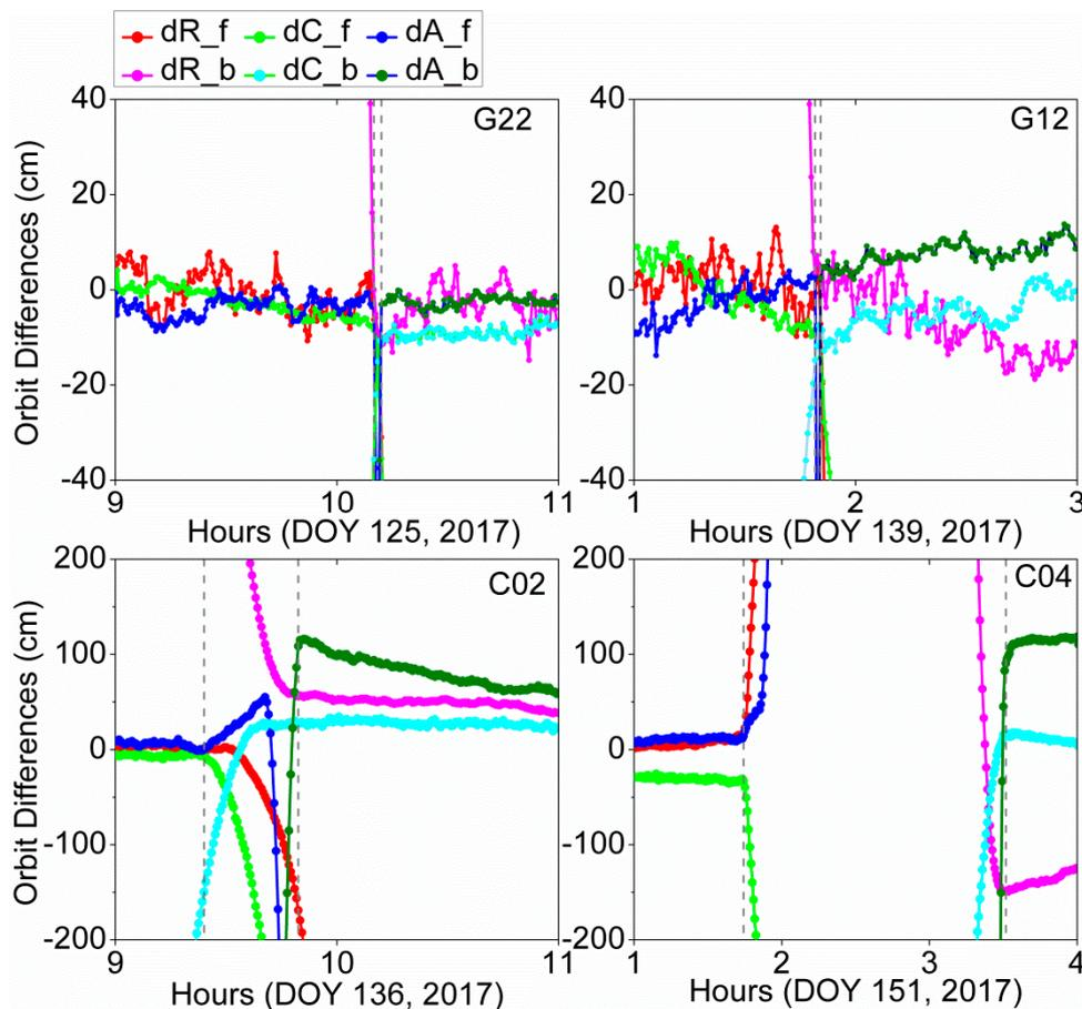
**Figure 7.** Orbit differences between the RPPP solutions and the forward and backward integration orbits for G22, G12, C02 and C04 around maneuvers. The vertical dashed lines indicate the detected start and end time of maneuver events.
