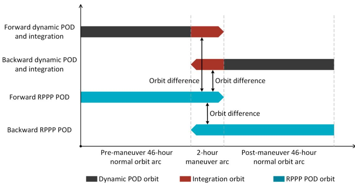
**Figure 6.** Computation and comparison strategy for the maneuvering satellites.
