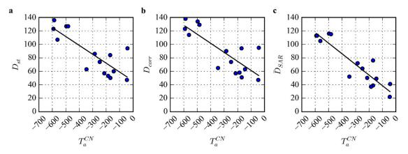
**Figure 17.** Scatterplots of the cumulative negative air temperature compared to the ice season duration (ISD) obtained from the coastal observations (**a**), maximum (**b**) and spatial-mean (**c**) ISD from the satellite data.
