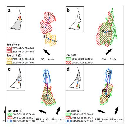
**Figure 6.** SAR-derived parameters of the ice drift in the Curonian Lagoon. (**a**) Drift of two ice floes observed on 4 April 2005; (**b**) drift of an ice floe on 28 March 2009; (**c**) drift of the first ice floe on 28 February and 2 March 2015; (**d**) drift of the second ice floe on 28 February and 2 March 2015. Labeled points indicate the polygon centroids, lines represent the linear distance between them, and the arrows indicate an average wind speed and direction.
