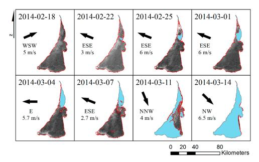
**Figure 9.** The ice cover retreat in the Curonian Lagoon in the winter of 2013–2014 under the prevalence of easterly and northerly winds. The red color indicates the ice cover boundary, the blue color shows water, the labels and arrows show the wind speed and direction.
