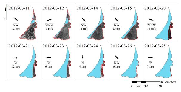
**Figure 8.** The ice cover retreat in the Curonian Lagoon in the winter of 2011–2012 under the prevalence of northwesterly winds. The red color indicates the ice cover boundary, the blue color shows water, the labels and arrows show the wind speed and direction.
