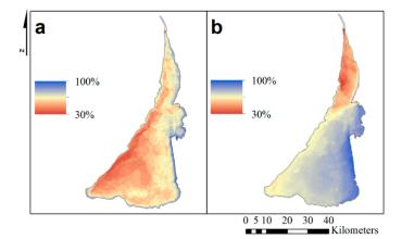
**Figure 13.** The spatial variations of the ice cover extent during (**a**) ice formation and (**b**) ice melting periods. The colors represent the percentage of ice observations during these periods, i.e., blue color in (**a**) shows the areas where the ice starts to form first, while the red color in (**b**) shows the areas where the ice melts first.
