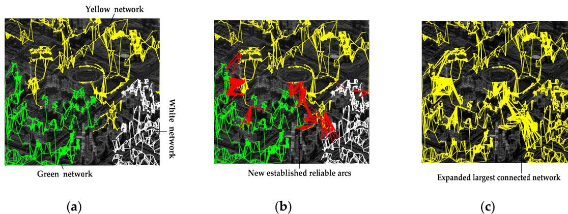
**Figure 8.** The process of establishing the largest connected network. (a) The main isolated networks after network adjustment; (b) establishing reliable arcs among the main isolated networks; (c) the expanded largest connected network.
