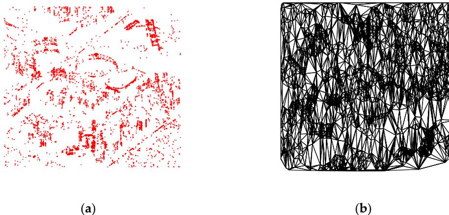
**Figure 6.** SPSCs and the first-tier network (a) SPSCs marked with red solid points; (b) first-tier network constructed by Delaunay triangulation.
