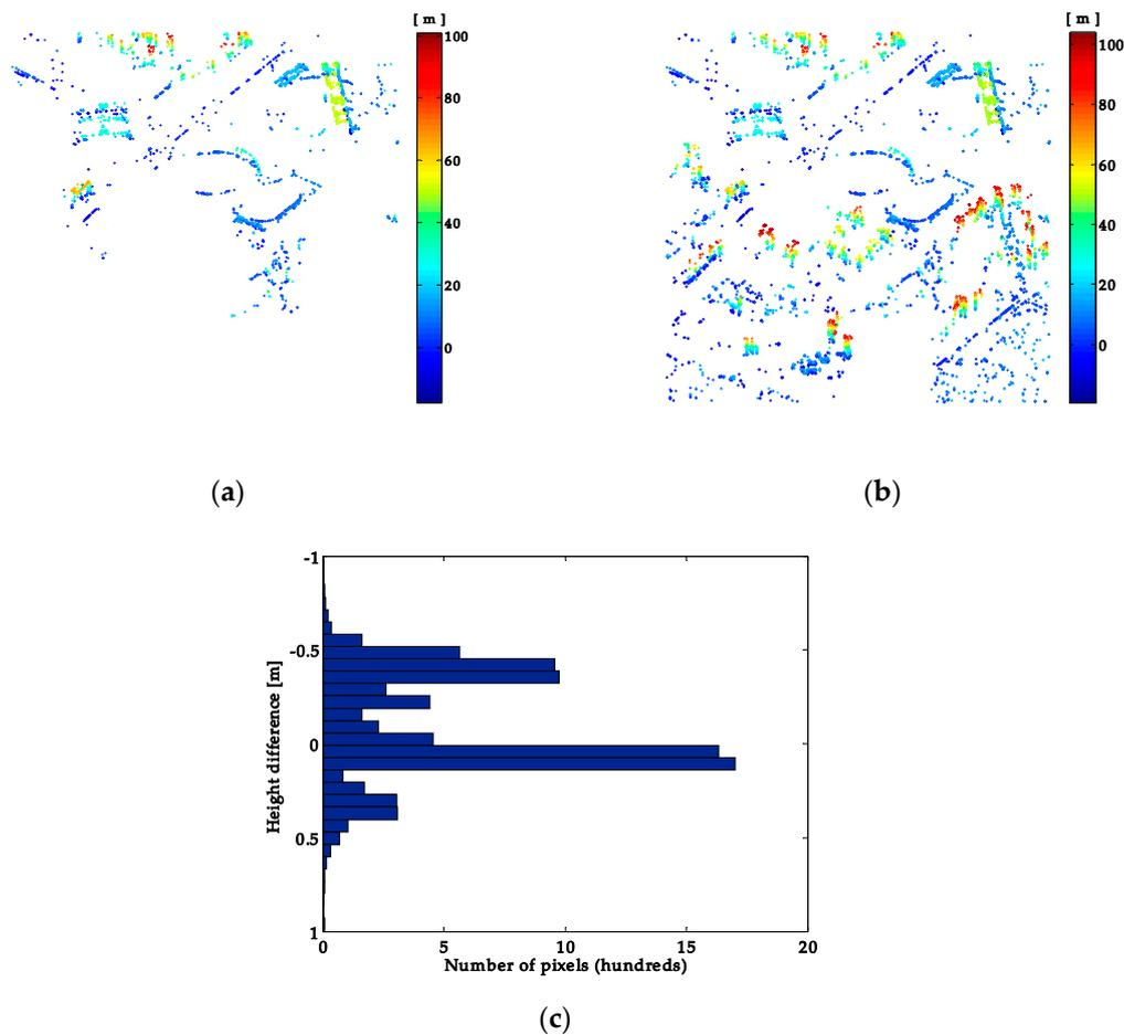
**Figure 10.** Estimated height of reliable SPSs and height difference histogram. (a) Estimated height of SPSs in the original largest connected network by ND-WLS estimator; (b) estimated height of SPSs in the expanded largest connected network by ND-WLS estimator; (c) the histogram of height difference between the height retrieved by ND-WLS estimator and WLS estimator.
