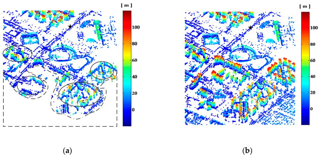
**Figure 11.** Estimated height of merged PSs. (a) Estimated height of merged PSs by traditional two-tier network; (b) estimated height of merged PSs by novel two-tier network.
