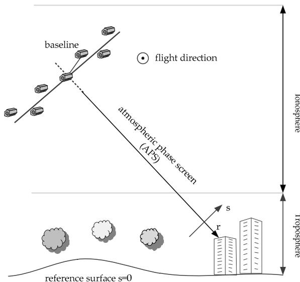
**Figure 1.** Multipass synthetic aperture radar (SAR) geometry in the range–elevation plane. The coordinate  $s$  is referred to as elevation. The satellite flies into the plane and looks to its right.
