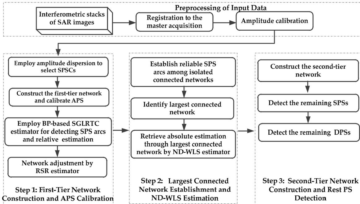
**Figure 2.** Flowchart of the new approaches for robust and efficient detection of persistent scatterers (PSs). Abbreviations: SPS, single persistent scatterer; DPS, double persistent scatterer; SPSC, SPS candidate; APS, atmospheric phase screen; BP, Beam-Forming; SGLRTC, sequential generalized likelihood ratio test with cancellation; RSR: residue-to-signal ratio; ND-WLS, network decomposition weighted least square.
