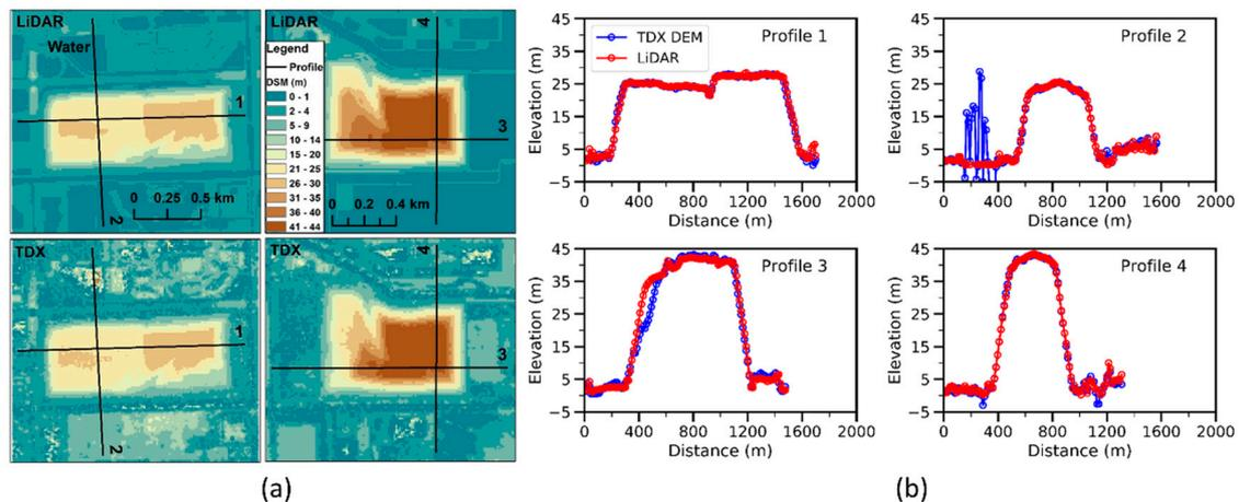
**Figure 5.** (a) TDX DEM of 12 m pixel size and corresponding LiDAR DSM of two trash mounds for profile analysis. Note that the TDX DEM image shows more noise than LiDAR DSM, especially in water bodies. (b) Elevation profiles extracted from TDX DEM and LiDAR DSM for two trash mounds.
