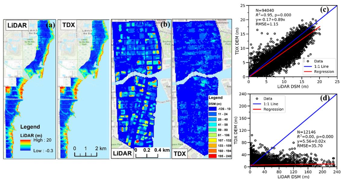
**Figure 8.** (a) LiDAR DSM and TDX DEM for the mangrove forest area along the east coast of South Florida. (b) LiDAR DSM and TDX DEM for downtown. Note that the TDX DEM represents the change of mangroves well, while the TDX DEM does not capture many high-rise buildings present in the LiDAR DSM. Linear regression between LiDAR DSM and TDX DEM elevations for the mangrove (c) and downtown (d) areas.
