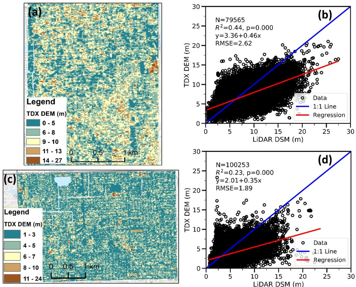
**Figure 10.** (a) TDX DEM for a sparse residential area, (b) scatter plot of LiDAR DSM and TDX DEM elevations for the sparse residential area, (c) TDX DEM for a dense residential area, and (d) scatter plot of LiDAR DSM and TDX DEM elevations for the dense residential area.
