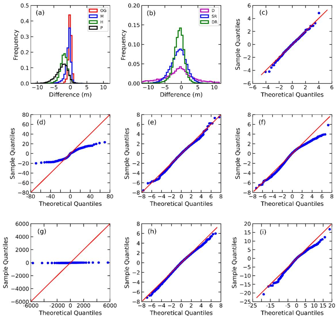
**Figure 7.** (a) Histogram of elevation differences between TDX DEM and LiDAR DSM in open ground (OG) and mangrove (M), hammock (H), and pine (P) forest areas. (b) Histogram of elevation differences between TDX DEM and LiDAR DSM in downtown (D), sparse residential (SR), and dense residential (DR) areas. Q-Q plots for open ground (c), mangrove forest (d), hammock forest (e), and pine forest (f), downtown (g), sparse residential (h), and dense residential (i) areas.
