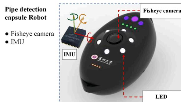
**Figure 4.** The appearance of the capsule robot.
