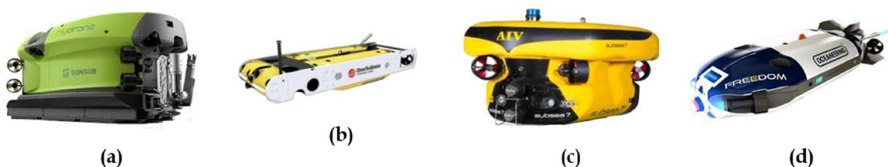
**Figure 5.** Some examples of Seabed-Hosted Vehicles (SHVs): (a) SAPIEM Hydrone-R [87]; (b) One-Subsea and SAAM Sabertooth [89]; (c) Subsea-7 AIV [86]; and (d) Oceaneering Freedom ROV [88].
