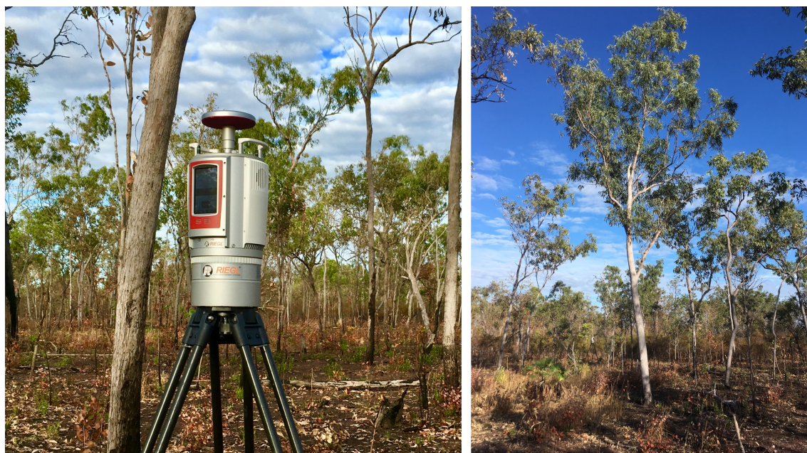
Figure 2. Site conditions at the time of the LiDAR surveys. Occlusion from the grass layer was minimal due to the effects of a fire one month prior.
