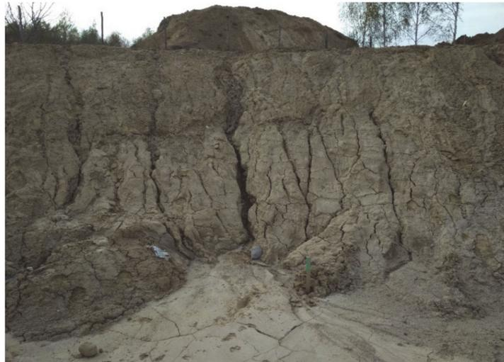
**Figure 3.** Rills and gullies caused by surficial runoff in silty soil as seen on-site.
