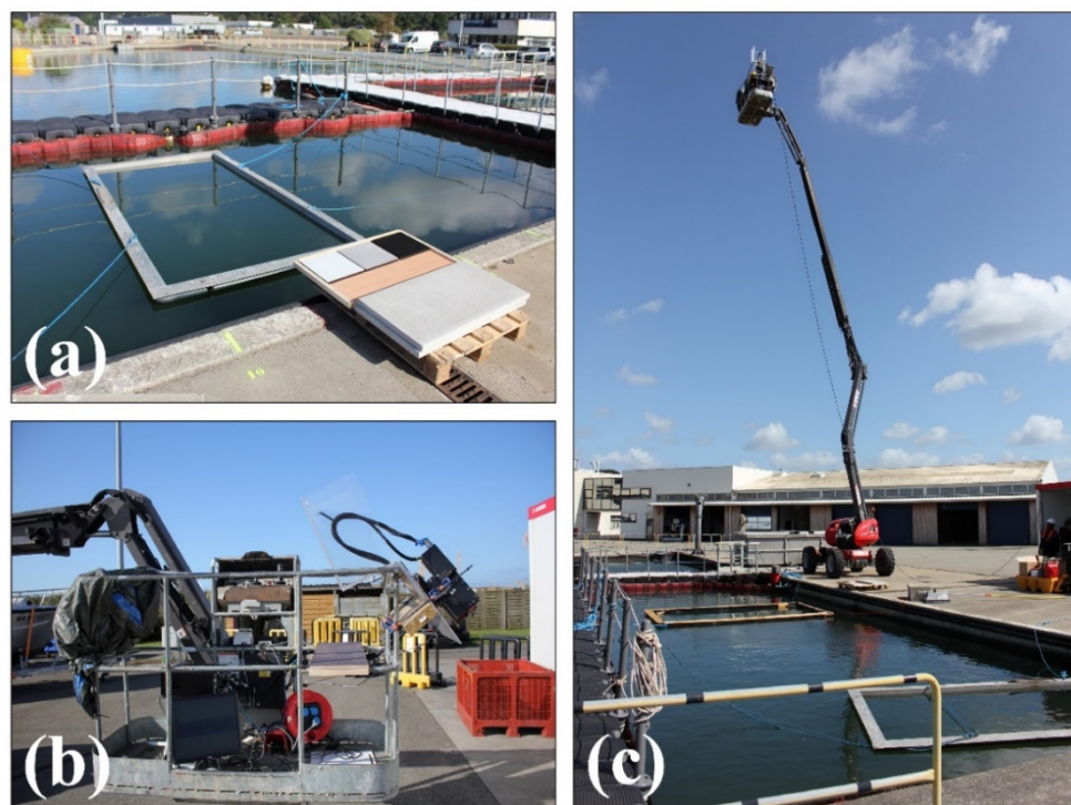
Figure 1. (a) Process of spilling of hazardous noxious substance (HNS) in a marine pool; (b) two hyperspectral cameras capable of observing visible and near-infrared (VNIR) and shortwave infrared (SWIR) wavelengths. (c) Location of the cameras at 12 m height using a lift.
