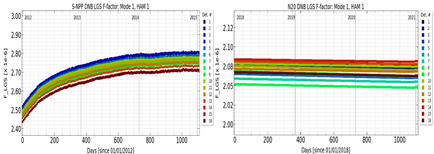
**Figure 12.** SNPP and NOAA-20 VIIRS DNB F-factor comparisons in the case of LGS mode-1 at HAM-1. DNB 16 detectors are plotted in different colors.
