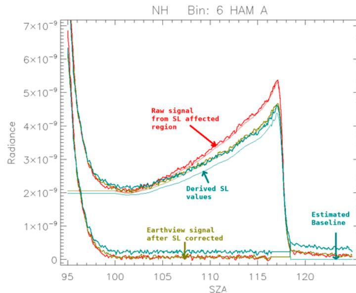
**Figure 10.** An illustration of stray light correction in bin-6: three detectors are presented in different colors. For each detector, the top noisy curve represents its raw signal. The smooth curve underneath the raw signal is its stray light estimate. After stray light correction, the signal is shown at the bottom.
