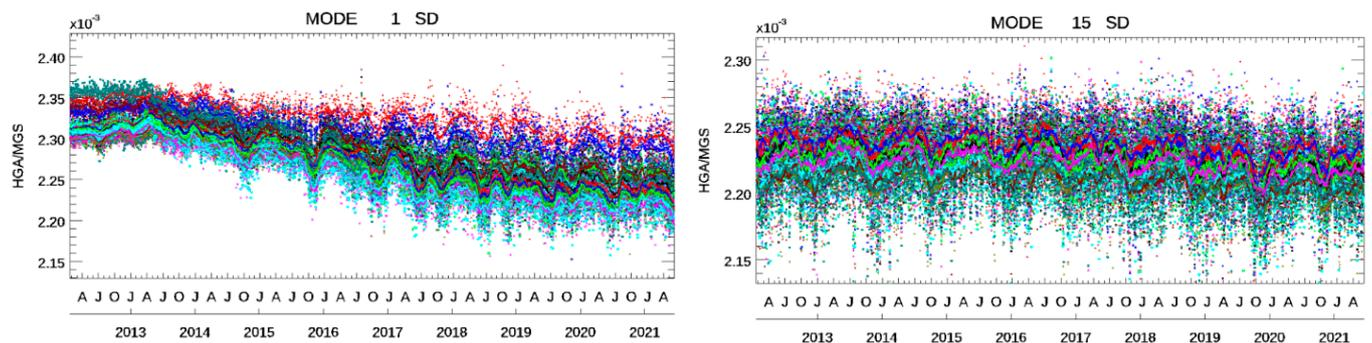
**Figure 5.** Ratio trend of DNB high-to-middle using SD *dn* signals at two aggregation modes (mode-1 and mode-15). Different colors are used to plot the DNB 16 detectors.
