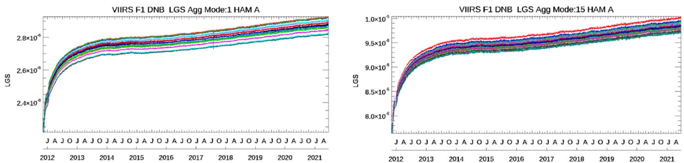
**Figure 3.** DNB daily averaged LGS F-factor trending at two aggregation modes (mode-1 and mode-15). Different colors are used to plot the DNB 16 detectors.
