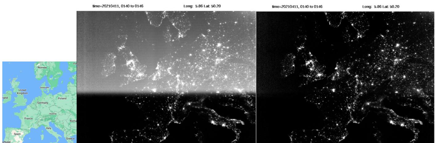
**Figure 11.** SNPP DNB images from 11 April 2021, 1:40 GMT. Images before/after stray light correction are located middle and right, respectively.
