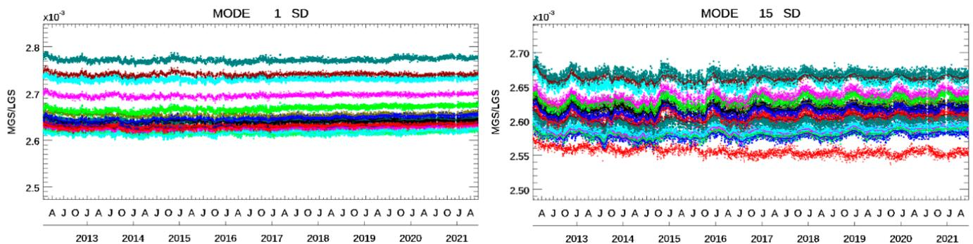
**Figure 4.** Ratio trend of DNB middle-to-low using SD *dn* signals at two aggregation modes (mode-1 and mode-15). Different colors are used to plot the DNB 16 detectors.
