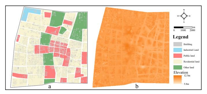
Figure 3. (a) Buildings extracted from GF-2 data and land-use type in the study area; (b) modified DEM based on buildings.
