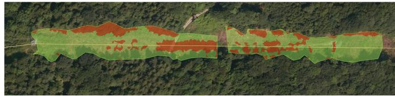
**Figure 9.** Overlap between the areas of detected encroaching vegetation (red) and the clearance areas (green).
