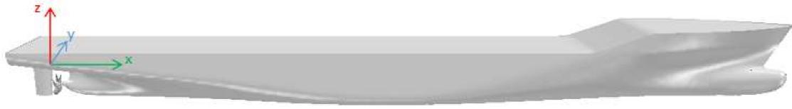
**Figure 3.** Geometry of the KCS hull with KP505 propeller.
