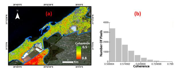
**Figure 10.** An excellent final coherence map result is shown based on the C-band Sentinel-1 data with values ranging from 0.5 to 0.8 (a) and its associated histogram (b).
