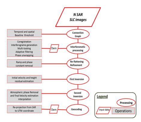
Figure 3. Flowchart of SBAS-DInSAR processing steps.
