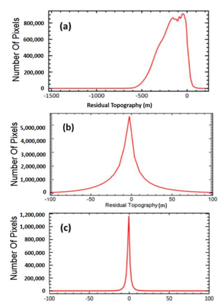
Figure 8. Statistics of estimated residual topography: (a) for ALOS-2 interferograms by using the SRTM data, which showed average residual topography equal to -100 m and high standard deviation equal to 70 m; (b) the average residual topography and standard deviation reduced by increasing the wavelet number; (c) for Sentinel-1 interferogram with average residual topography to almost 0 m with a standard deviation equal to 13.5 m.
