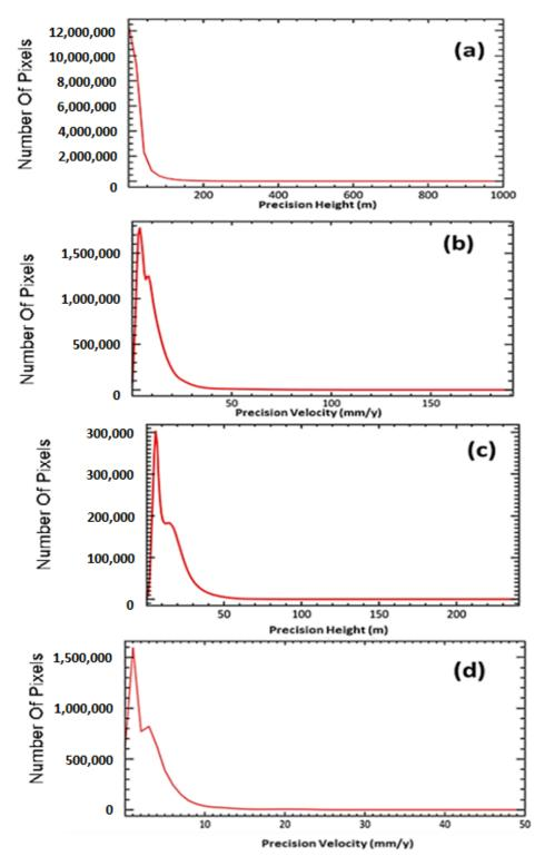
**Figure 9.** (a) Statistics histograms of precision height and (b) the corresponding height precision for ALOS/PALSAR-2 data. (c) Representative histograms of Sentinel-1 data precision height and (d) the corresponding precision velocity.
