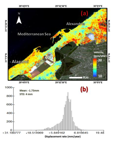
**Figure 14.** (a) The estimated mean displacement velocity of Alexandria and Alagami Cities using the Sentinel-1 data from August 2017 to September 2020 with coherence threshold of 0.4; (b) the corresponding histogram distribution of the derived displacement velocity rates.
