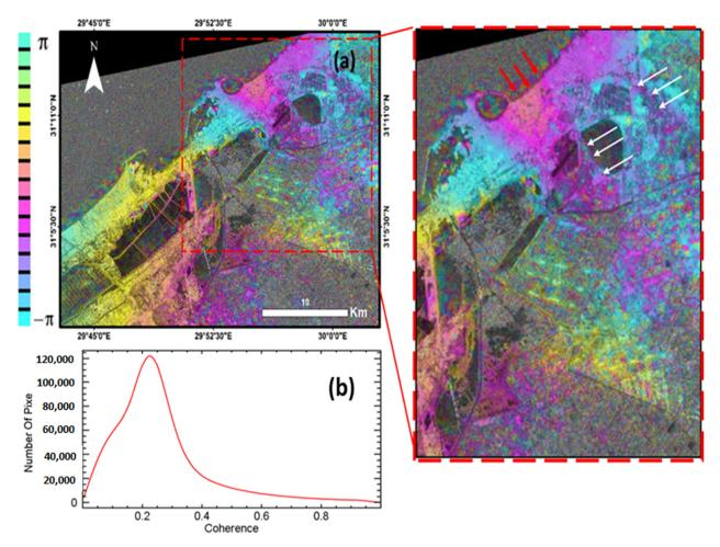
**Figure 6.** (a) Wrapped ALOS-2 low coherent interferogram showing errors during the flattening sub-step; white arrow indicates systematic residual fringes that could have been caused by strong orbital inaccuracy or issues with some parameter settings, while red arrows indicate strong atmospheric artifacts and phase jumps. (b) Histogram representing the coherence value of interferogram with a mean coherent value of 0.15.
