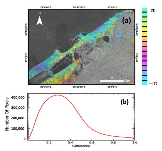
**Figure 7.** Wrapped Sentinel-1 interferogram with low coherence. The cause is the very large temporal and normal baseline between the two acquisitions used to make the interferogram (**a**). The histogram illustrates the coherence value between two interferogram pairs (master 15 December 2018 and Slave 10 June 2019) (**b**).
