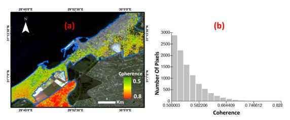
**Figure 11.** The final coherence coverage of ALOS-2 data which is very poor with average coherence values of about 0.6, standard deviation of 0.04 and about 80% of Alexandria City show no coherent data (**a**) and its associated histogram (**b**).
