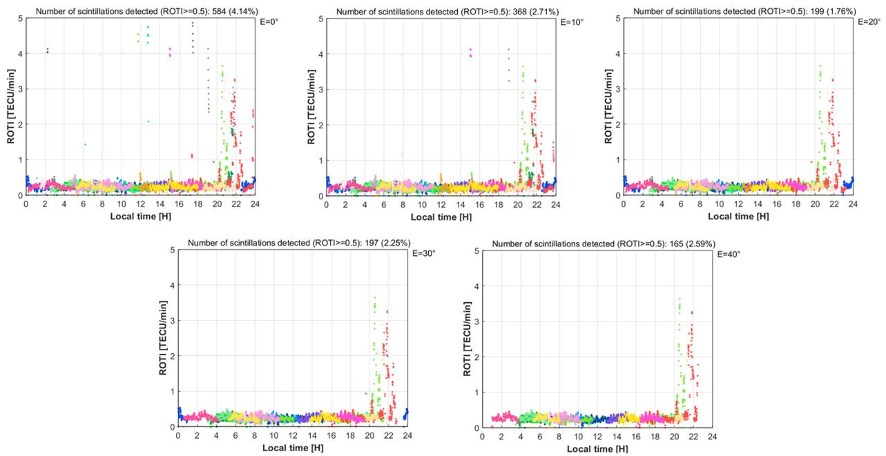
**Figure 6.** Comparison of scintillation events with different elevation thresholds at Hanoi station (Vietnam) on 24 October 2015. It can be seen that the different threshold elevations give very different amounts of detectable irregularities, with the threshold elevation of 20° eliminating most of the multipath noise while keeping essentially the required number of observations.
