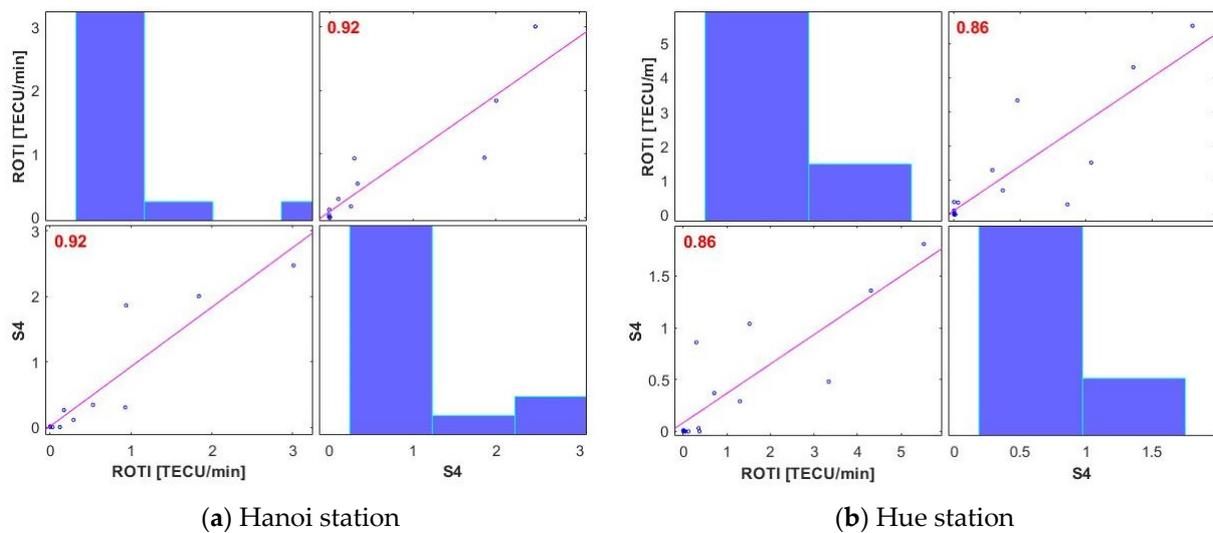
**Figure 5.** Correlation coefficient (percentage of electronic disturbances compared to the total of the observations) between ROTI and S4 at Hanoi (a) and Hue (b) stations during the period of 15–28 March 2015. The similarity between these two indices at Hanoi station is 0.92, slightly higher than at Hue station with 0.86. Both of these indices demonstrate good conformity between ROTI and S4 indices.
