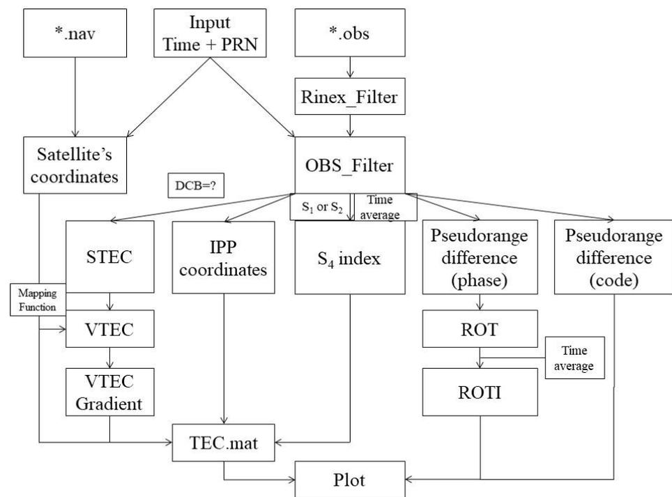
**Figure 3.** Flowchart of the ionosphere software tool. The input data are the observation and navigation files of the RINEX data. The output results include certain ionospheric parameters with the aim of detecting disturbances in the ionosphere that affect the GNSS measurements.
