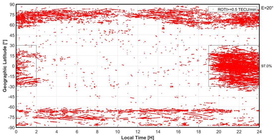
**Figure 14.** Temporal distribution of global ionospheric irregularities, showing clear differentiation by latitudinal region. In the low-latitude regions, about 97.0% of ionospheric irregularities detected appear during the evening hours, i.e., from 19 LT to 2 LT the next day. The remaining 3.0% only occur scattered during different times of the day.
