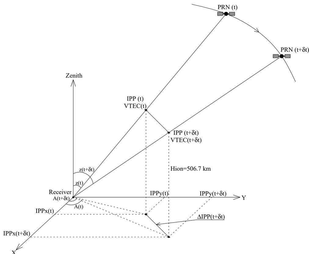
**Figure 2.** Principle of determining VTEC gradient from the movement of satellites using the projection of IPP on horizontal plane. This is calculated from the displacement of the satellites after each epoch, meaning it describes both temporal and spatial gradients of VTEC.
