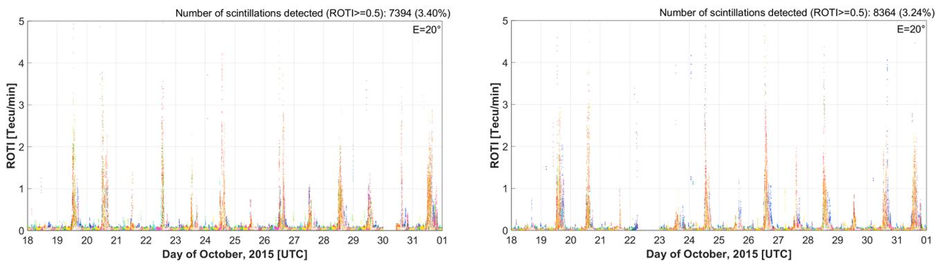
**Figure 8.** ROTI observations during the period of 18–31 October 2015 at Hue (left) and CUSV (right) stations. It can be seen that ionospheric disturbances occurred densely during this period. These was also one of the periods when the Sun was most active during the last solar cycle and almost all GNSS stations in the Southeast Asia region were strongly affected.
