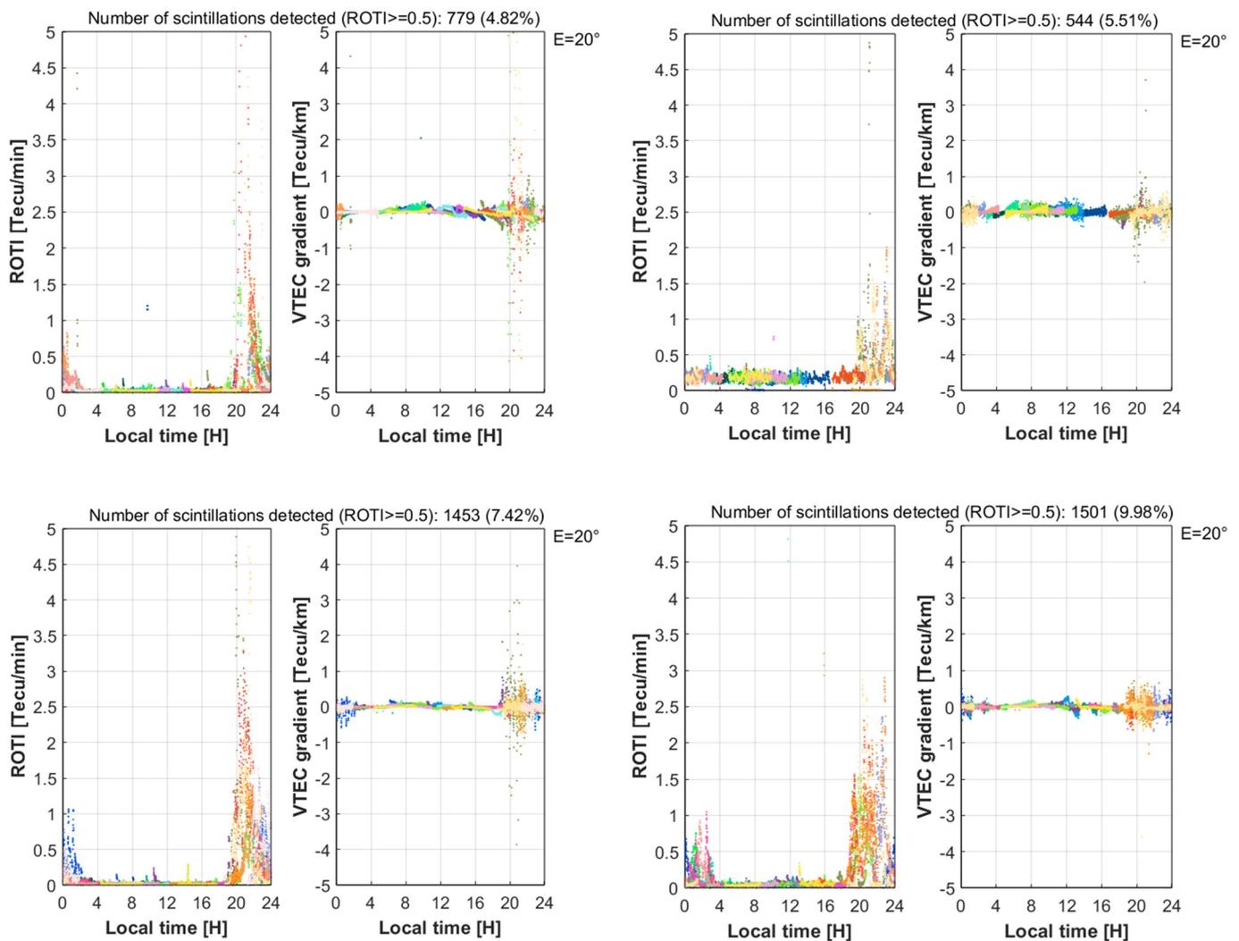
**Figure 9.** Ionospheric irregularities including ROTI and VTEC gradient values at BAKO station on 19 October (**top-left**), HCM station on 20 October (**top-right**), CUSV station on 26 October (**bottom-left**), and at HUE station on 31 October (**bottom-right**). While the ROTI shows the temporal distribution of ionospheric disturbances, the VTEC gradient indicates both spatial and temporal distributions of plasma ionospheric irregularities.
