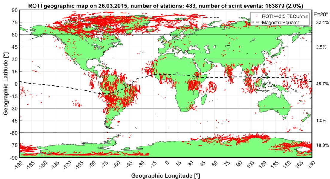
**Figure 13.** Spatial distribution of global ionospheric irregularities (only  $\text{ROTI} \geq 0.5$  TECU/min are displayed). The total number of ionospheric irregularities detected (163,879) corresponds to approximately 2.0% of the total number of observations obtained on this day. The regions most likely to be affected by ionospheric disturbances are South America and the Arctic.
