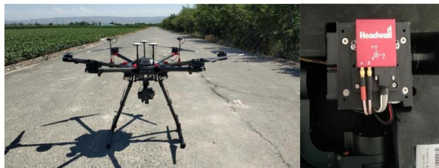
**Figure 2.** DJI Matrice 600 series aircraft equipped with the GPS and a sensor (left). The Nano-Hyperspec sensor (right).
