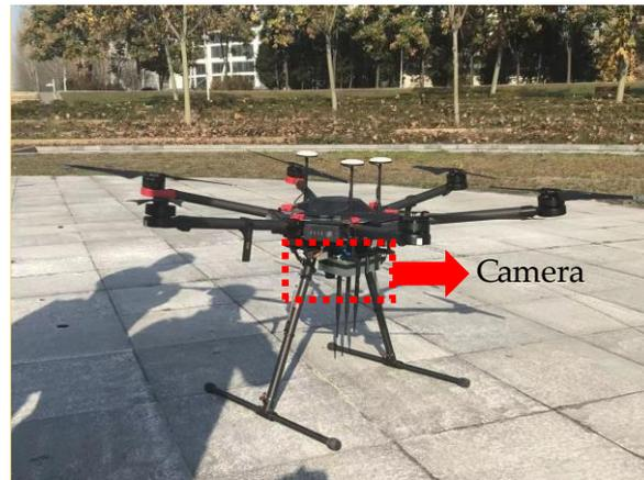
**Figure 9.** Homemade UAV platform based on DJI M600 and 1080P camera.
