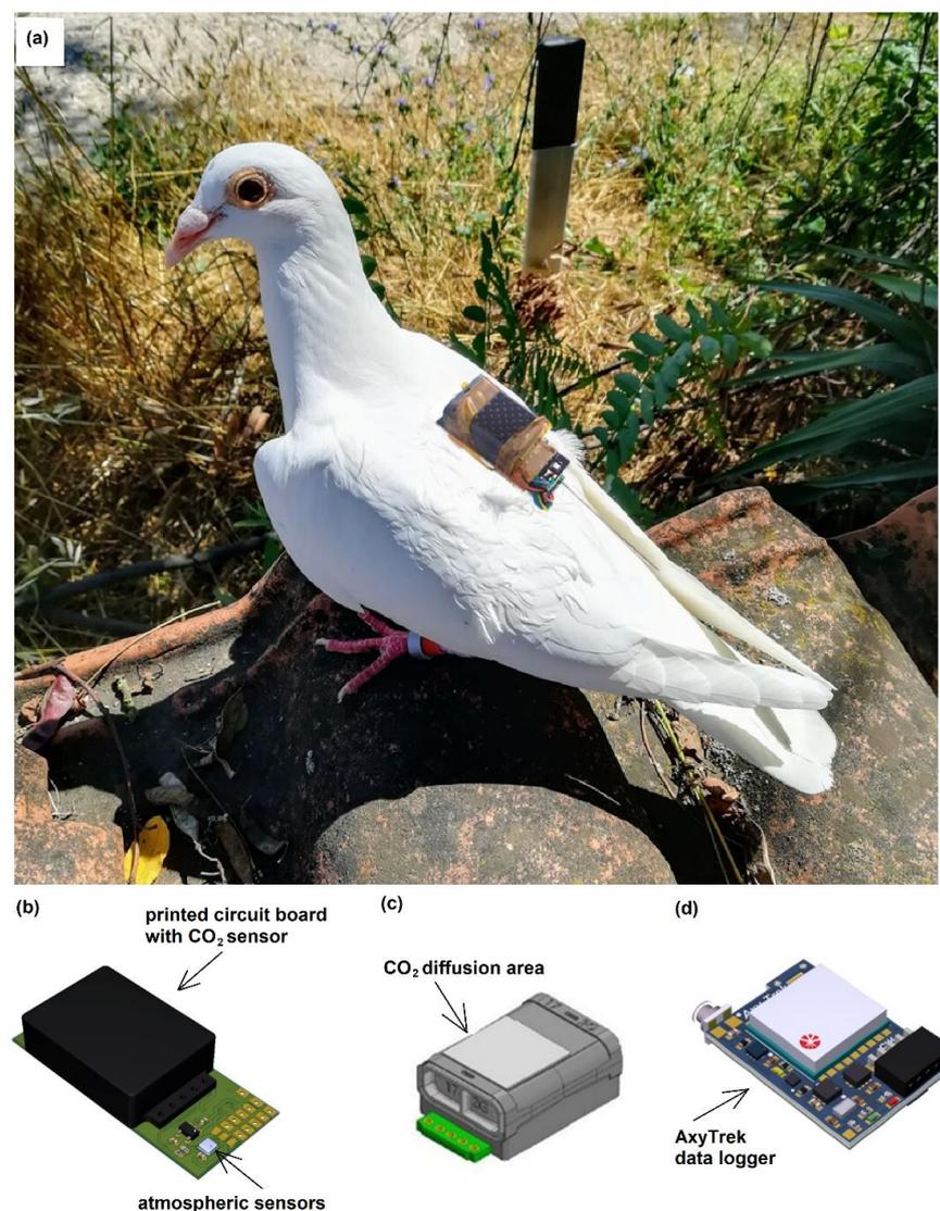
**Figure 1.** Photograph of the device attached on a homing pigeon (a), schematic view of printed circuit board with CO<sub>2</sub> and atmospheric sensors (b), CO<sub>2</sub> sensor (Senseair Sunrise, Senseair AB, Delsbo, Sweden) with the gas diffusion area represented by the white membrane (c), and AxyTrek data logger (d).
