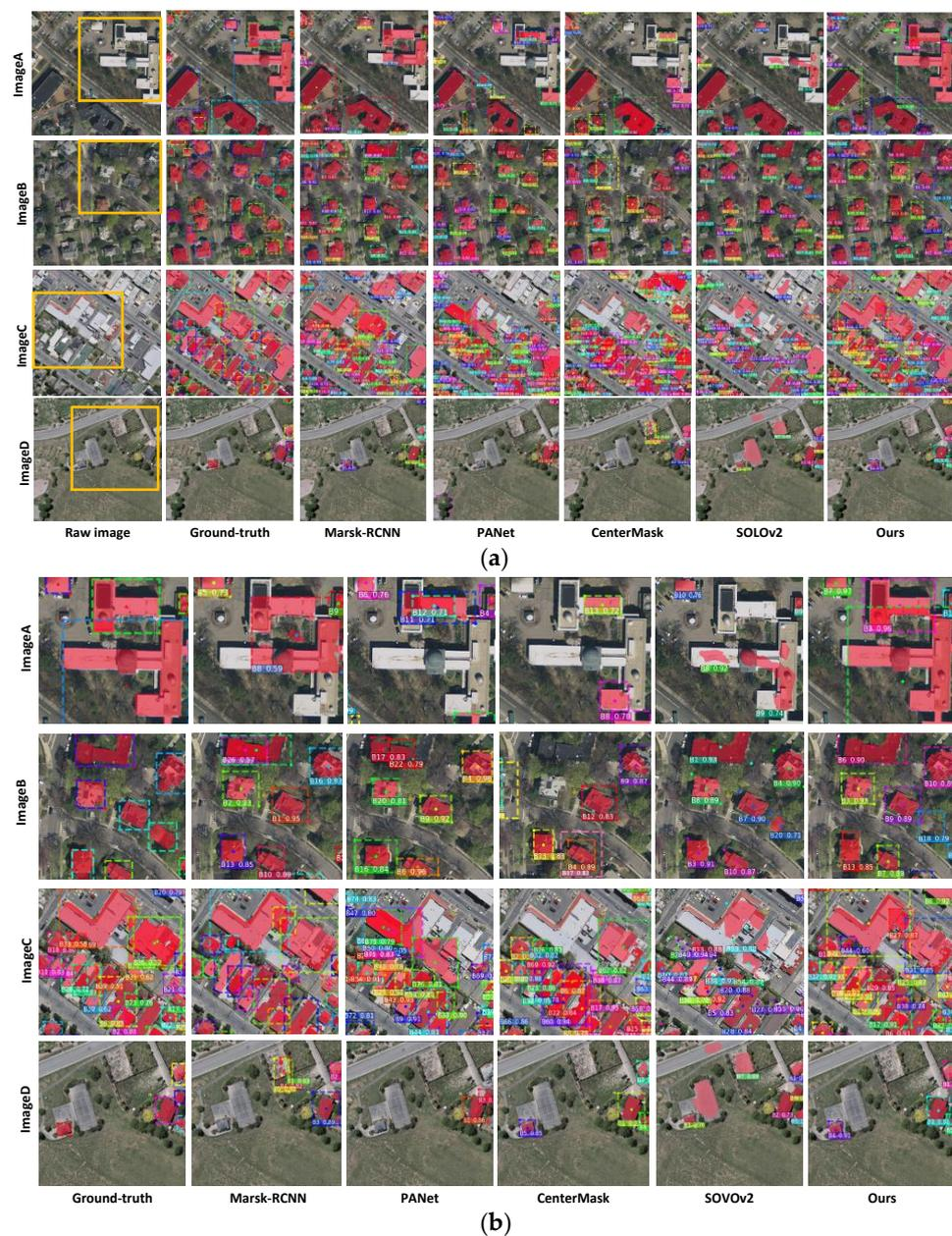
**Figure 12.** (a) presents the building instance segmentation results using different methods. The details in the yellow rectangles are enlarged and closely inspected in (b), where the segmentation results are marked with red for comparison, and the detection result is marked with a random color. The dotted rectangle denotes the predicted bounding box, and the dot denotes the geometric center of the bounding box.
