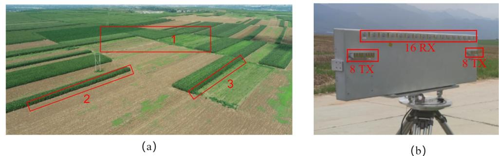
**Figure 8.** Experiment scene and system. (a) Low-lying and wide open fields. (b) GB-SAR system with 16 TX and 16 RX.
