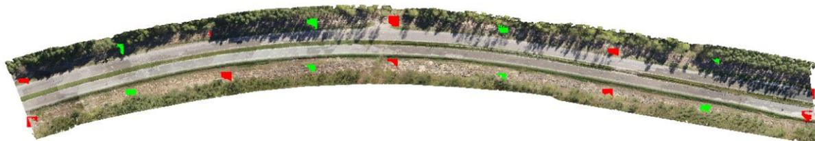
**Figure 10.** The curved highway with four segments and irregular GCP distribution.
