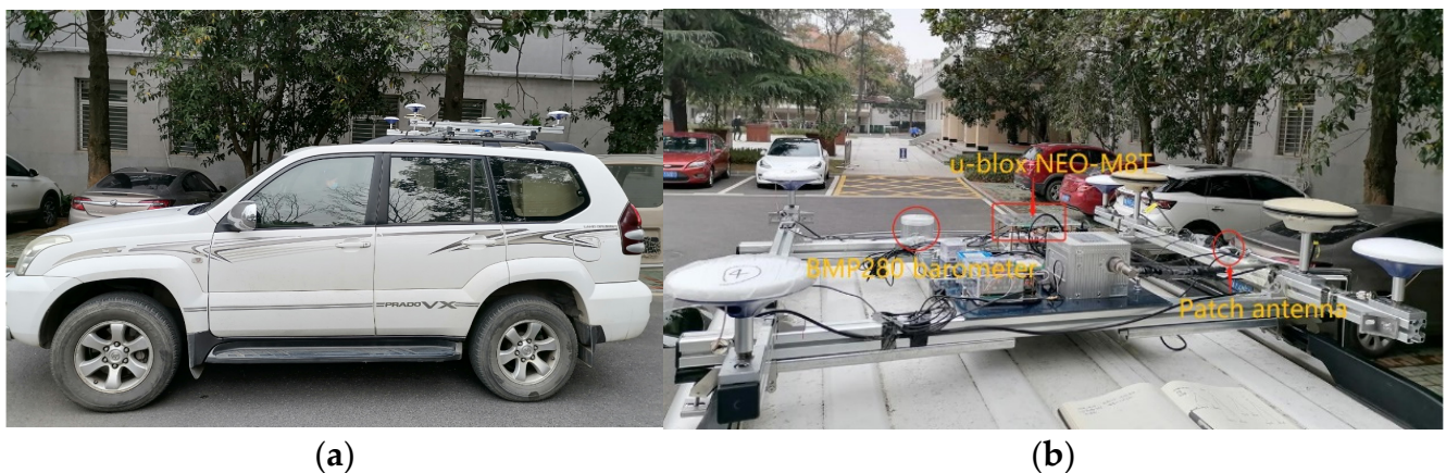
Figure 11. The mobile station hardware equipment site for kinematic vehicle experiment, including four geodetic GNSS receivers and antennas, NovAtel SPAN-FSAS GNSS/INS system, low-cost NEO-M8T receiver with a patch antenna, and a BMP280 barometer: (a) the experimental vehicle; (b) equipment setup diagram.
